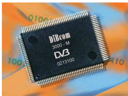
Figure 1 DIB3000-M demodulator chip
