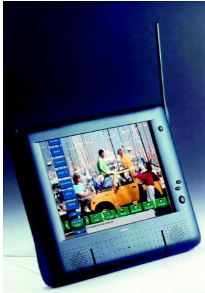
Figure 3 Nokia's Media Screen combines mobile DVB-T reception with GSM to provide mobile broadband delivery capabilities.
