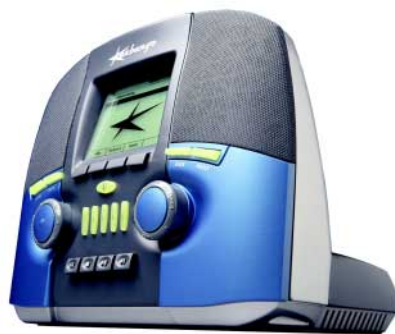
Figure 5 By means of a wireless link from an Internet-connected PC, the Kerbango receiver can “tune in” to Internet radio stations. The unit also includes an FM receiver.
