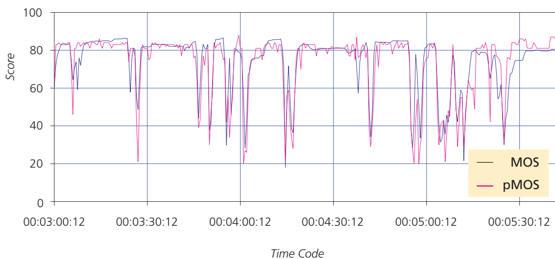
Figure 5 The objective (pMOS) and subjective (MOS) quality of a sequence affected by transmission errors.
