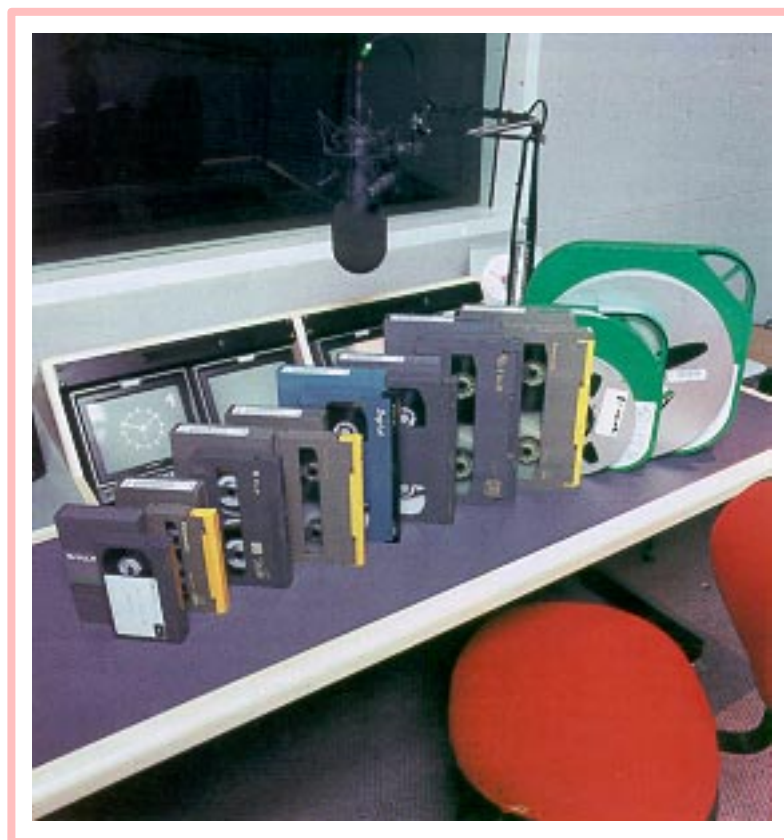
Figure 1 Typical range of tapes currently encountered by broadcasters, from the 1-inch open-reel format to samples of the many sizes and types of cassette-based formats.
