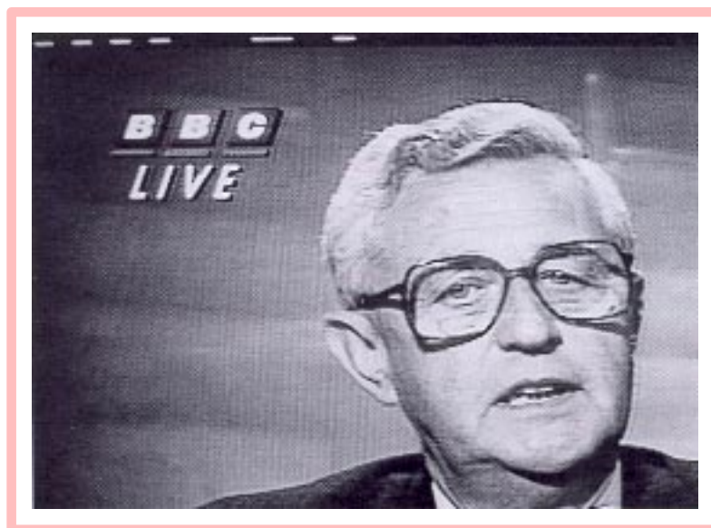
Figure 5 Off-screen photograph from an under-scanned monitor showing the delay code in the vertical blanking interval.
