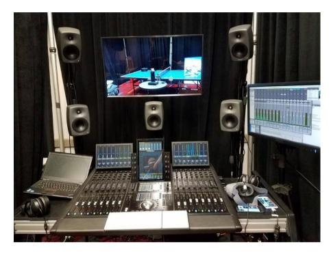
Figure 6: An example of a monitoring system for the simultaneous production of SBA for VR and linear TV content. The workstation features a 7.1.4 loudspeaker system, an HMD for VR monitoring, and a DAW.
