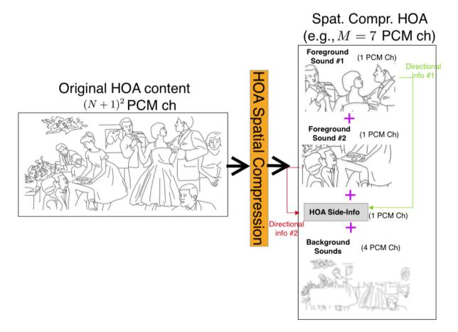
Figure 7: Graphical representation of the HOA spatial compression. The HOA sound scene is analysed and decomposed in foreground and background components and HOA side info.
