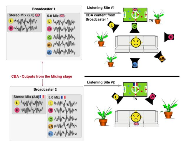
Figure 2: Delivery and reproduction of Channel Based Audio Content
