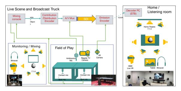
Figure 10: Audio Workflow for simultaneous NGA, VR, and 360 video production
