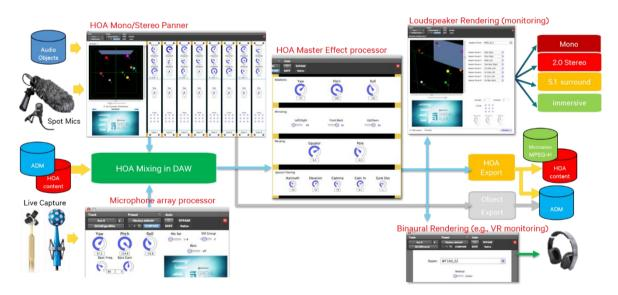
Figure 5: An example of a 3D audio production workflow based on HOA and the Qualcomm® 3D Audio tools suite [30]
