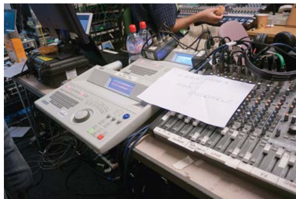
Photo 2 A view of the "NetMix" operator position showing the sub mixer, the shortcuts and instructions to leave the sustaining feed faded up when the court was off air
