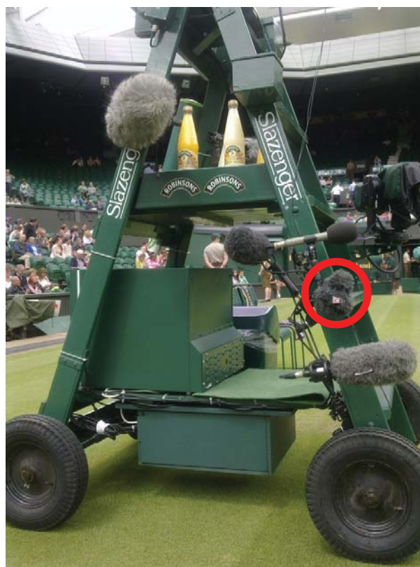
Photo 1 A crossed pair of Neumann km100s (along with other BBC paraphernalia) mounted on the umpire's chair on Wimbledon centre court
