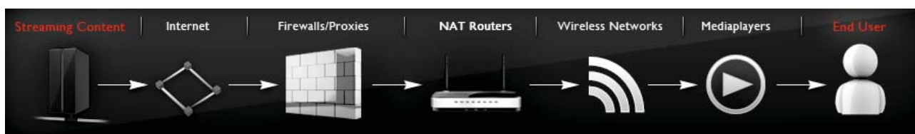
Figure 1 Many things on the way from source to end-user can increase RTT and packet loss
