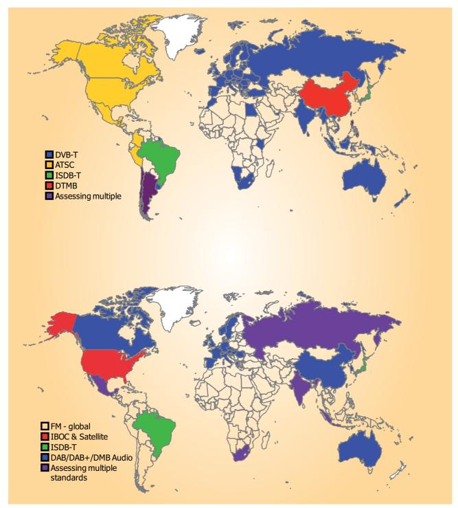
Figure 2 Global standards for *(upper)* digital TV and *(lower)* radio
