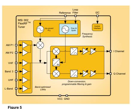
Mirics reconfigurable multi-standard FlexiRF<sup>™</sup> tuner
