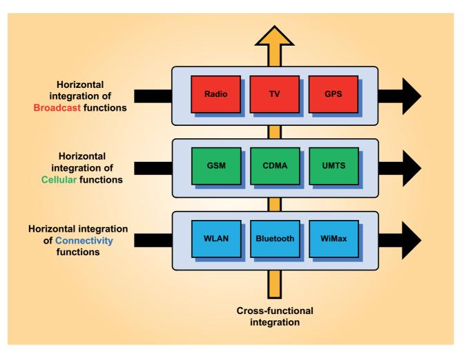
Figure 3 Radio integration architectures for consumer electronics devices
