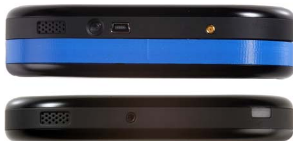
Figure 4 Comparison of thickness between the original device and the Openmokast prototype
