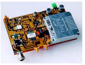
Figure 7 Nujira HAT Power Modulator integrated with PA
