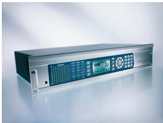
Example of an ISDN and Audio over IP fixed end unit
