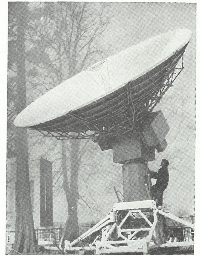
A 21 ft. diameter air-transportable dish reflector assembly, supplied to G.E.C.-A.E.I. (Electronics) Ltd., manufacturers of the earth terminal part of the satellite communications system "Skynet".
