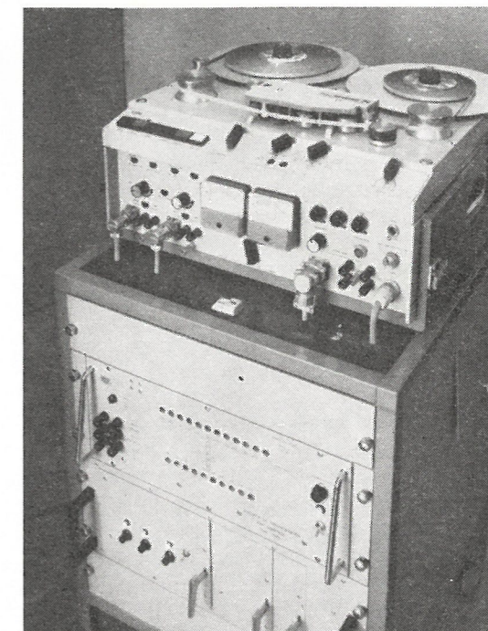
Sound tape-machine associated with the system for synchronisation by means of counting, enabling it to work synchronously with a television tape-machine.
