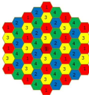
Figure 3: Ideal hexagonal network with frequency re-use N=4
