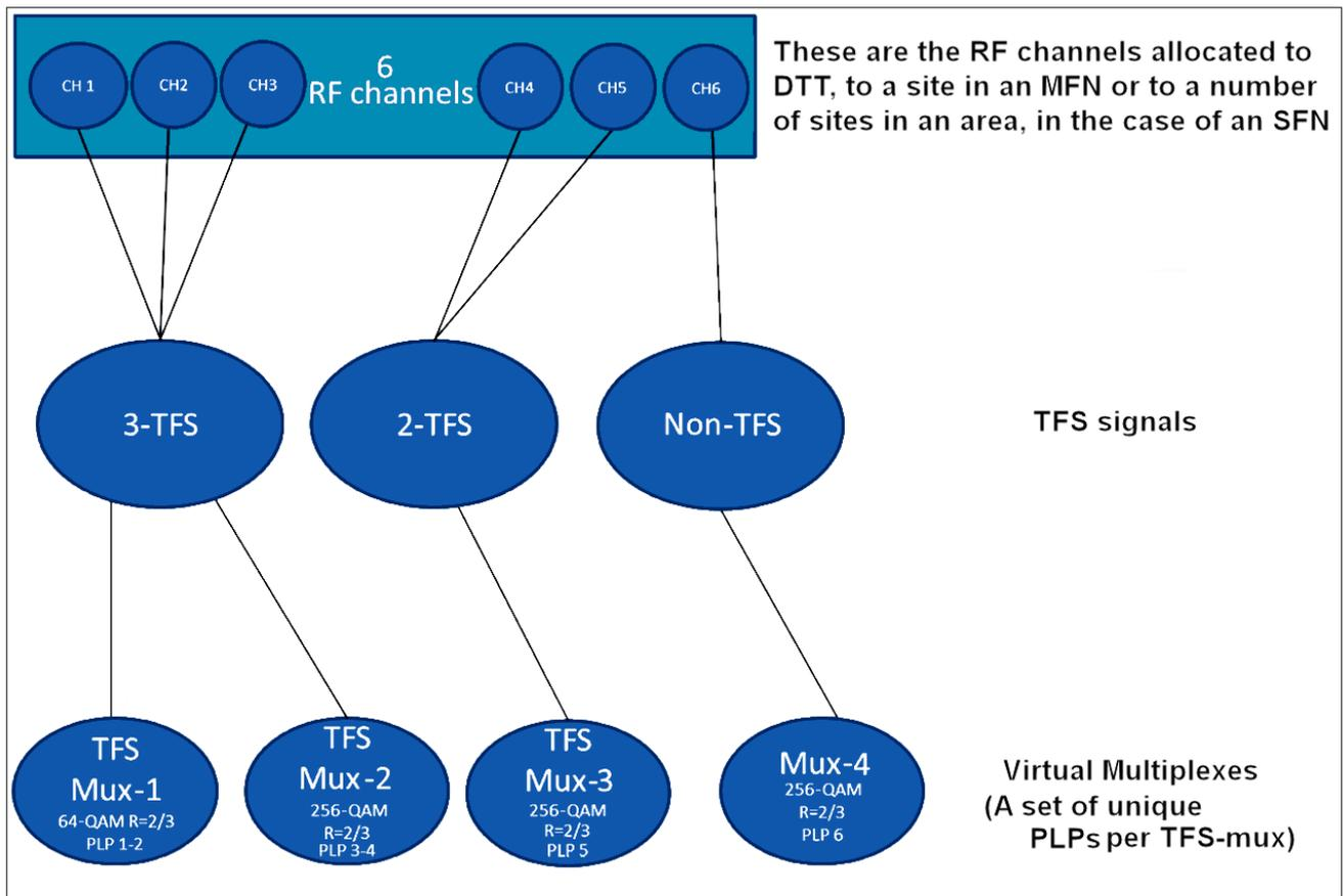
Figure 10: Example of 6 RF channels split into 3 different TFS signals
