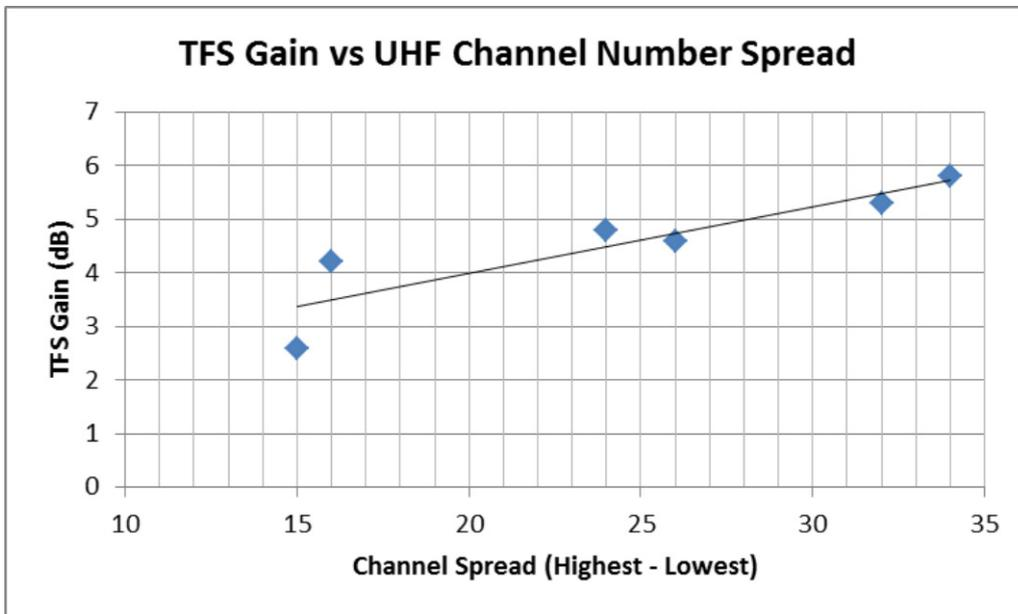
Figure 7: TFS-gain and channel spread
