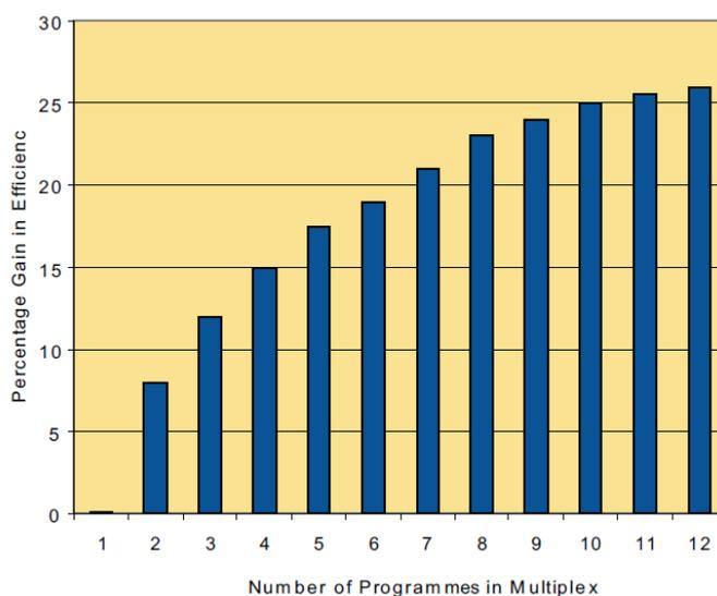
Figure 9: Efficiency gain<sup>4</sup> of statistical multiplexing
