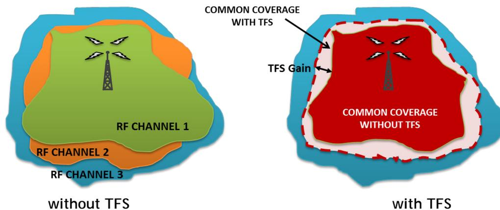
Figure 2: Example of area coverage for three RF channels in a DTT network
