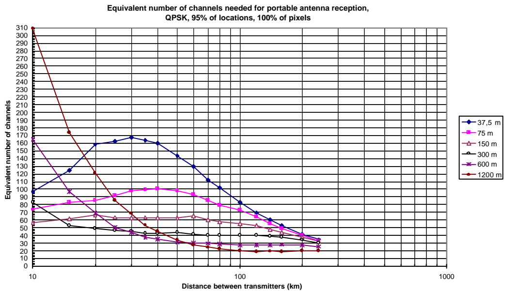
Figure C4: Equivalent number of channels needed for coverage with the same data capacity (20-24 Mb/s), for portable indoor antenna reception, using 64QAM, 16QAM or QPSK. Location probability: 95%, pixel coverage: 100%. Parameter: H_{\text{eff}} .
