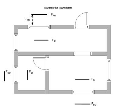
Figure E3: Field strength measurement points inside and outside a building
