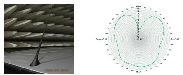
Figure C2: Quarter wave slant whip on car roof
