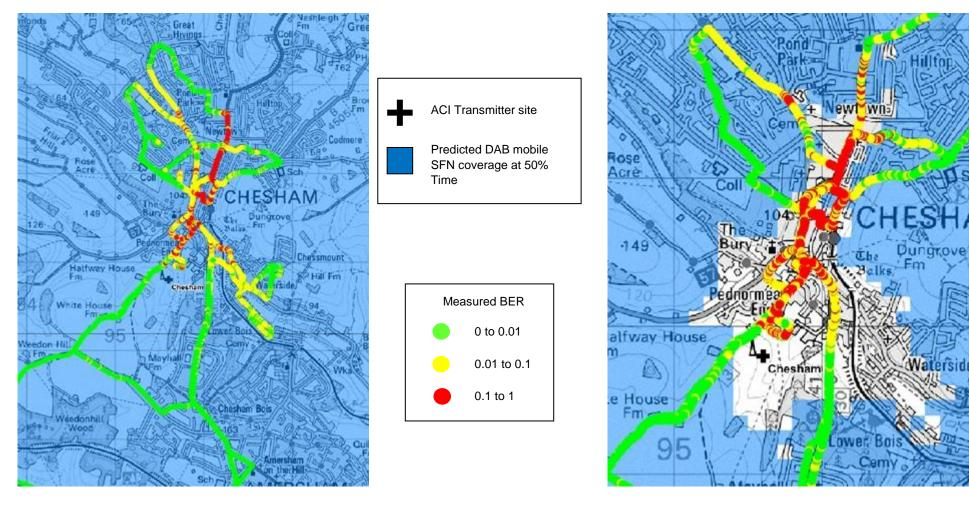
Figure 15: Predicted mobile coverage and channel 11D BER with No Adjacent Channel Interference
