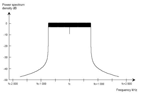
Figure 2: DAB transmission signal spectrum (1.536 MHz channel) (from ETSI Standard EN 300 401 [ETSI\_2])
