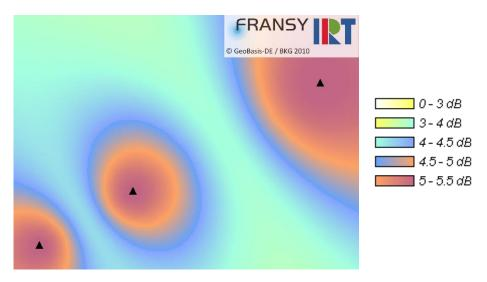
Figure G3: Standard deviation in a single frequency network
