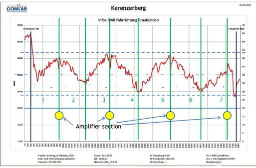
Figure J2: Sample measurement for minimum coverage criteria for DAB (courtesy of Comlab AG, measurements performed with a rooftop quarter wave antenna with k factor of 16 dB/m)
