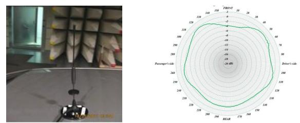
Figure C1: 'Ideal' Quarter wave monopole on car roof
