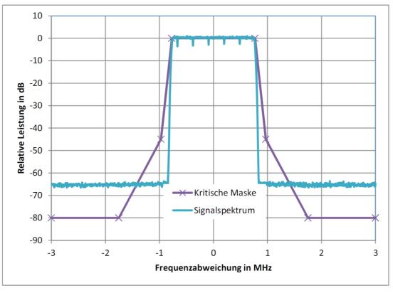
Figure 9: Undistorted signal considered in IRT studies [OS\_12]
