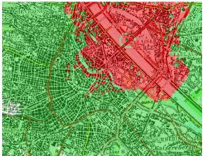
a) 100 m resolution prediction at 10 m a.g.l. and fixed height loss of 12.4 dB (Low Urban)
