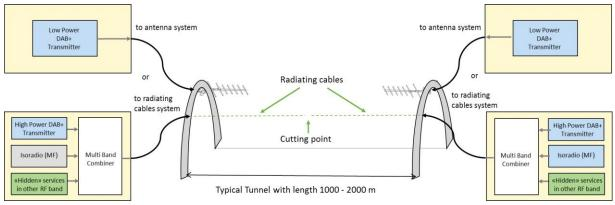
Figure J3: Radiating cable VS directive antenna
