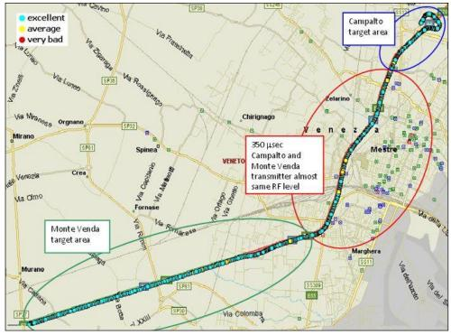
Figure H5: Audio quality measured travelling on highway
