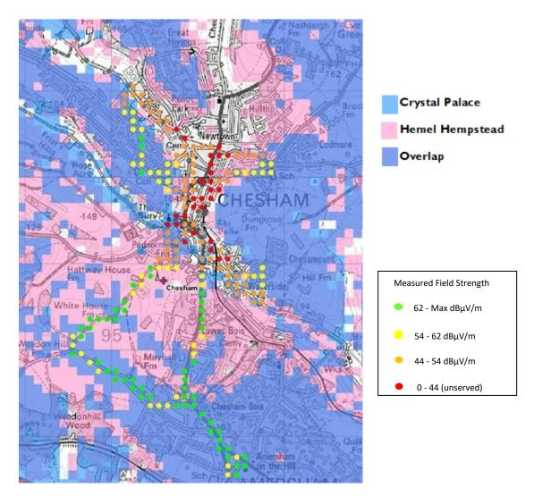
Figure 13: Predicted mobile coverage for channel 11D in Chesham from the two dominant servers, Crystal Palace and Hemel Hempstead (Gross transmitter coverage - No SFN gain). Drive survey measured Field Strength for channel 11D is also shown (measured at 1.5 m a.g.l. and averaged into 100 m pixels) The antenna pattern for the proposed channel 12B service from the Chesham site is shown in Figure I4.
