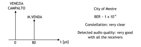
Figure H3: Relative delay in Mestre from the two transmitters in test
