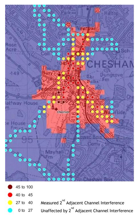
Figure 17: Predicted channel 11D mobile SFN coverage in Chesham before and after the channel 12B transmitter is brought to air at 100 W ERP compared with the Measured Field Strength Difference.
