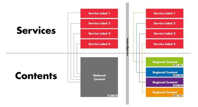
Figure K3: Scheme of the ensemble content before and after the reconfiguration
