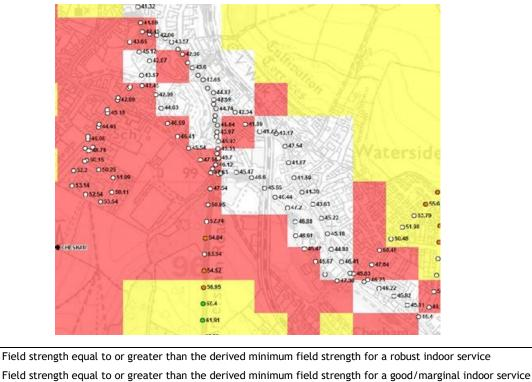
Field strength less than the derived minimum field strength for an indoor service
