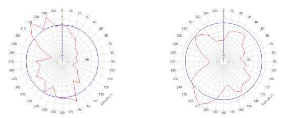
Figure C3: Typical in-glass antenna patterns
