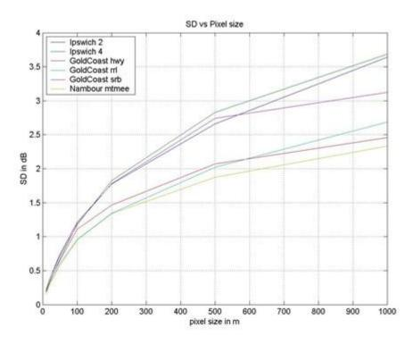
Figure F8: SD mean values vs pixel size for Lee filtered using 40 wavelengths and uncorrelated data samples
