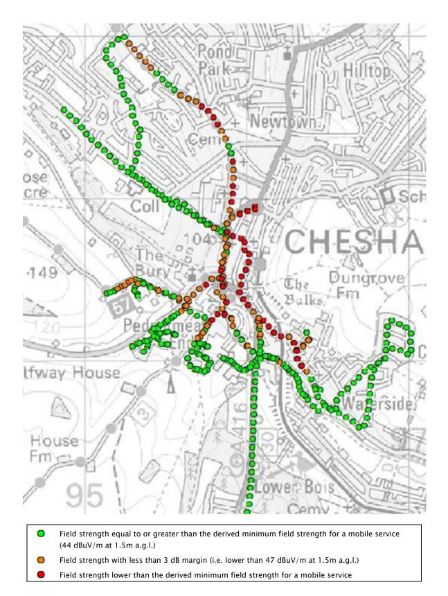
Figure 18: Measured field strength data for the channel 11D service in Chesham before any ACI but showing areas considered unserved for a mobile service.
