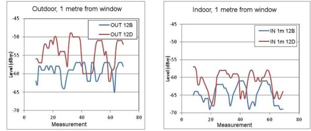
Figure E9: Indoor and outdoor signal measurements of channels 12B and 12D
