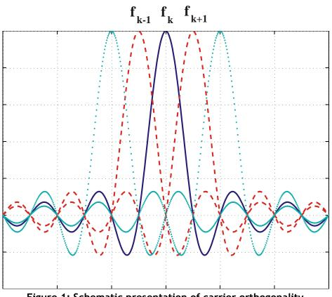
Figure 1: Schematic presentation of carrier orthogonality in an OFDM signal (after windowing)
