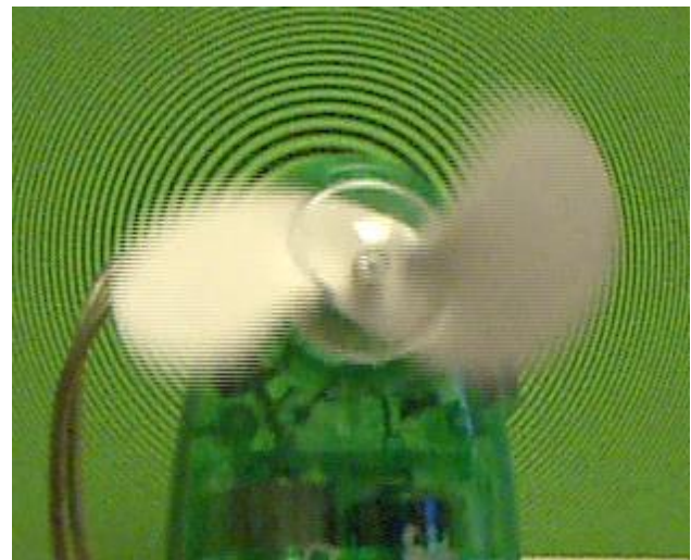
Figure 9 Rotating fan, rolling shutter
