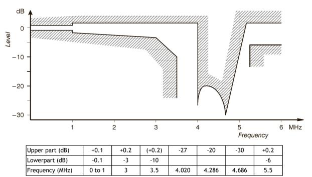
Fig. 2 - Luminance passband mask (SECAM)
