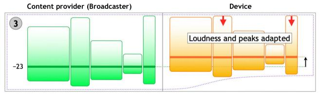
The device is used in a situation with limited playback gain and headroom and/or higher background noise; High quality True-peak limiting is performed where needed (see the two red arrows).
