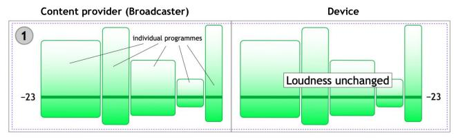
The device is used in a situation with sufficiently high playback gain and headroom as well as low background noise.
