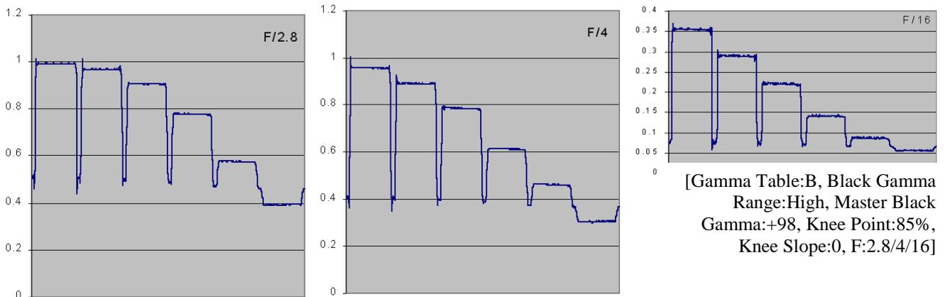
F/4 is probably not optimum exposure at standard gain, since the knee is already compressing the brightest patches somewhat. At F/2.8, the brightest patches are being significantly compressed, but are still easily discriminable. At F/16, the “black” patch is being compressed a little because the slope at black is not infinite, as is required for perfect colour analysis.
