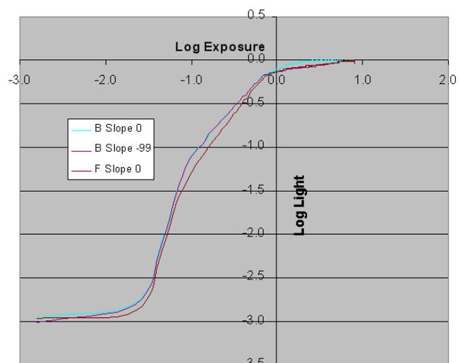
[Gamma Table:B/F, Black Gamma Range:High, Master Black Gamma:+98, Knee Point:85%, Knee Slope:-99/0, Gain:+18dB]
