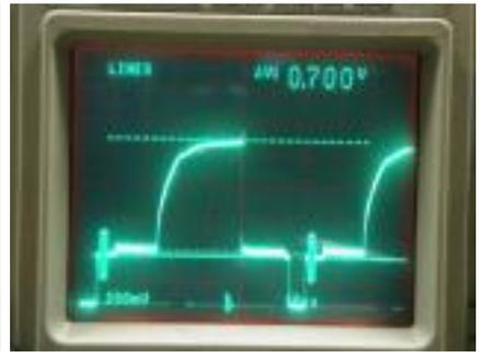
[Gamma Table:B, Black Gamma Range:High, Master Black Gamma:+98, Knee Point:85%, Knee Slope:0, Gain:+9dB]
