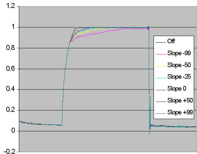
[Gamma Table:B, Black Gamma Range:High, Master Black Gamma:+98, Knee Point:85%, Knee Slope:-99/-50/-25/0/+50/+99, Gain:+18dB]
