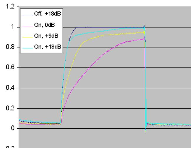
[Gamma Table:F, Black Gamma Range:High, Master Black Gamma:+98, Knee Point:85%, Knee Slope:0, Gain:0/+9dB/+18dB]
