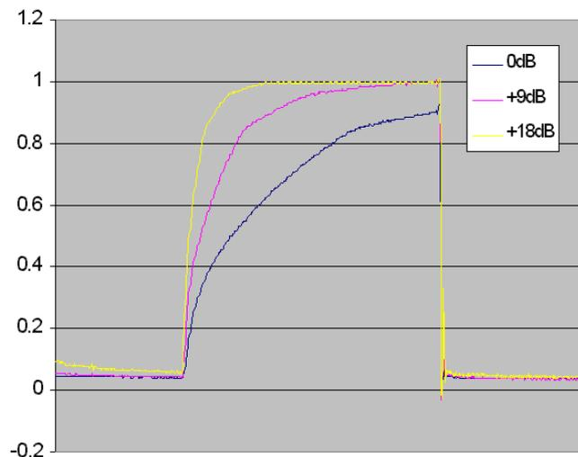
[Gamma Table:B, Black Gamma Range:High, Master Black Gamma:+98, Knee Point:85%, Knee Slope:0, Gain:0/+9dB/+18dB]
