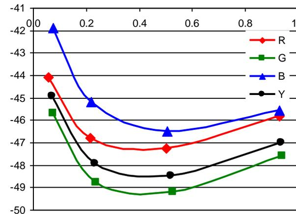
Figure 6 Noise levels, noise reduction=4 (a) 1080p (b) 720p
