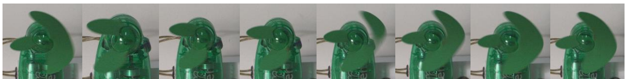
Figure 11, rolling shutter effect, rotating fan, 1/1000 shutter
