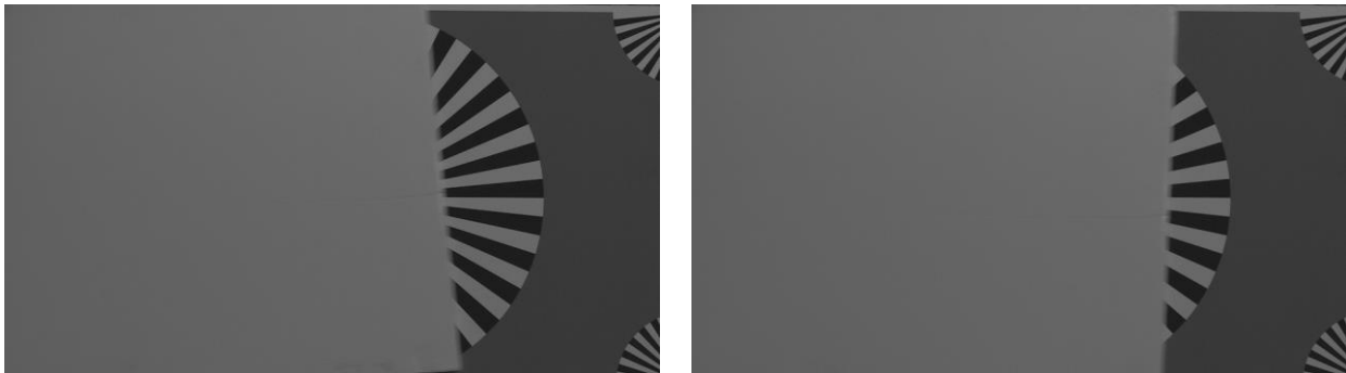
Figure 10, rolling shutter effect, (a) left to right motion (b) right to left motion
