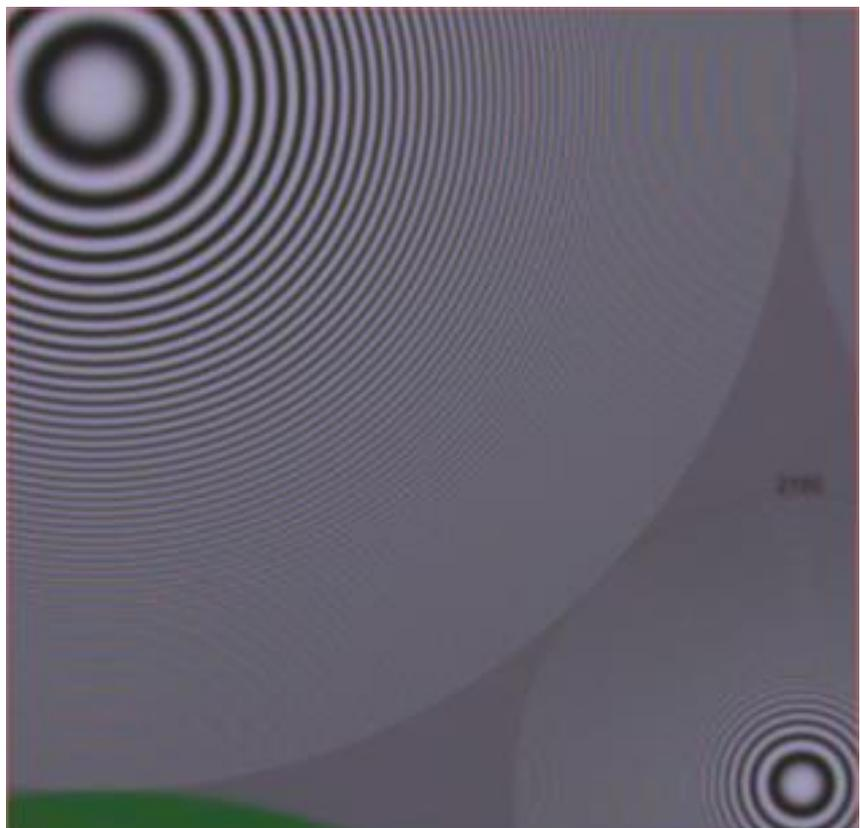
camcorder, with a 1920x1080 Bayer-patterned sensor, the coloured alias level is very similar. The result is not pleasing, and should not be considered suitable for use in HDTV production.
