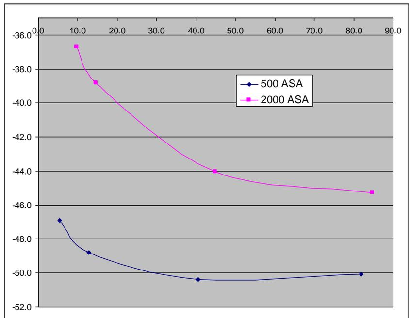
bits in linear and/or 10-bits in log. This is one disadvantage of recording video using a log curve rather than a conventional gamma curve with knee function to extend the contrast range, since the gamma curve makes more efficient use of the available bit-depth, delivering up to 6dB better noise performance on test.
