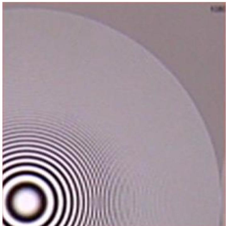
this is because the SD output is interlaced, and the down-conversion is correctly limiting the vertical to that admissible in an interlaced signal. However, since the HDTV image is not particularly sharp anyway and relatively free from aliasing, the down-conversion is actually rather good.
