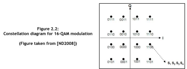
There are various ways of attributing the bits to the symbols. Best results are achieved if only one bit is changed when going from one symbol to the next closest symbol. In this way only one bit is mistaken when a symbol mismatch occurs with the next closest symbol. This coding is called Gray mapping. **Figure 2.2** shows a Gray mapping constellation.
