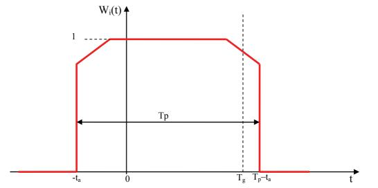
Figure 4.5: Weighting function  $w_i(t)$  (with an equalization interval EI starting at  $t = -t_a$ )
