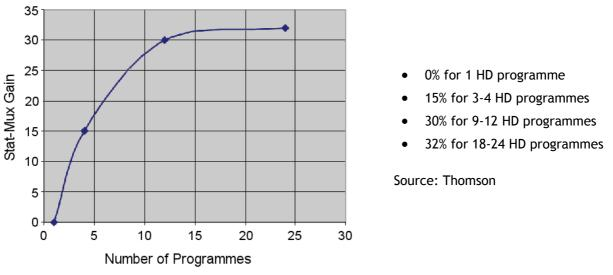
Figure 4.11: Statistical multiplex gain with MPEG-4 AVC
