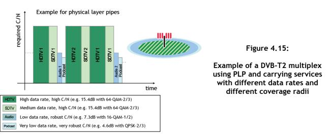
An example is given in **Figure 4.15** where four different classes of services (HDTV, SDTV, Audio Broadcasting and Data Broadcasting) are carried in one multiplex. Each of the services has a different data rate and a different coverage radius indicated in the Figure on the right hand side.
