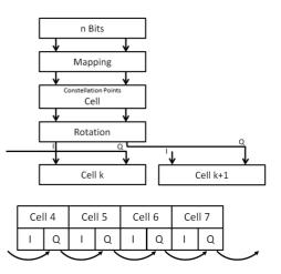
A cell is the result of mapping a later carrier. In contrast to DVB-T, mapping is not carried out after all interleaving processes but relatively early, after the error protection and after the bit interleaver. However, this is still followed by the cell interleaver, the time interleaver and the
