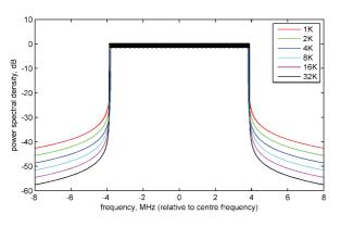
Figure 2.6: Theoretical DVB-T2 signal spectrum for guard interval fraction 1/8 (for 8 MHz channels and with extended carrier mode for 8k, 16k and 32k)
