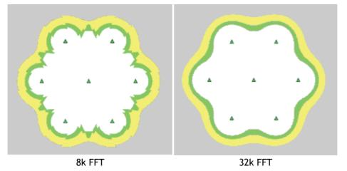
Figure 4.3: Comparison of the coverage areas for the 8k and the 32k FFT mode
