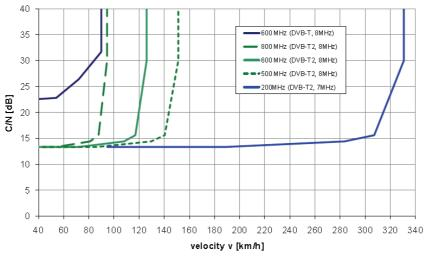
Figure 2.5: Required C/N for DVB-T and DVB-T2 as a function of the velocity of the mobile receiver, 8k FFT (from [AFM2010])
