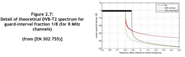
Because of its higher number of usable carriers the extended carrier mode has an increased data capacity as the normal carrier mode. **Table 2.16** gives the gain of the extended carrier mode for the different FFT modes.
