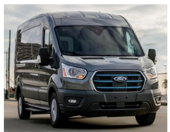
The e-Transit, with 198 kW (269 hp) engine and 68 kWh battery (75 kWh gross capacity). Range of up to 315 km.3 lengths, 2 heights, van versions, van with extended cab, chassis with single cab and a load volume ranging from 9.5 to 15.1 m3.
