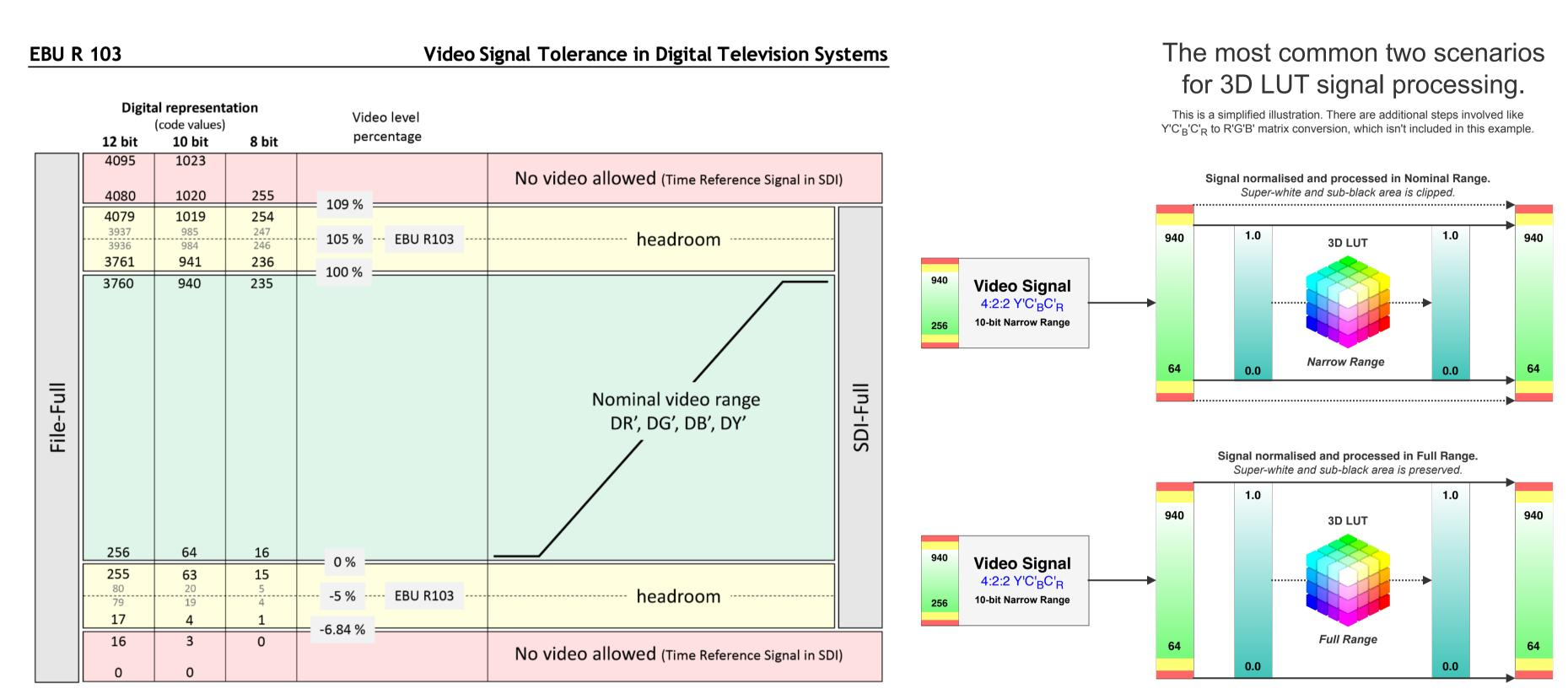
Figure 1: Typical signal levels for SDI
