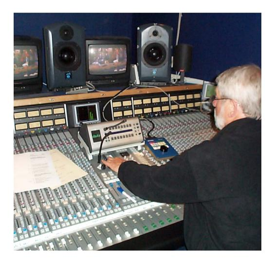
The remote control for the Dolby Multichannel Audio Tool used for monitor listening
