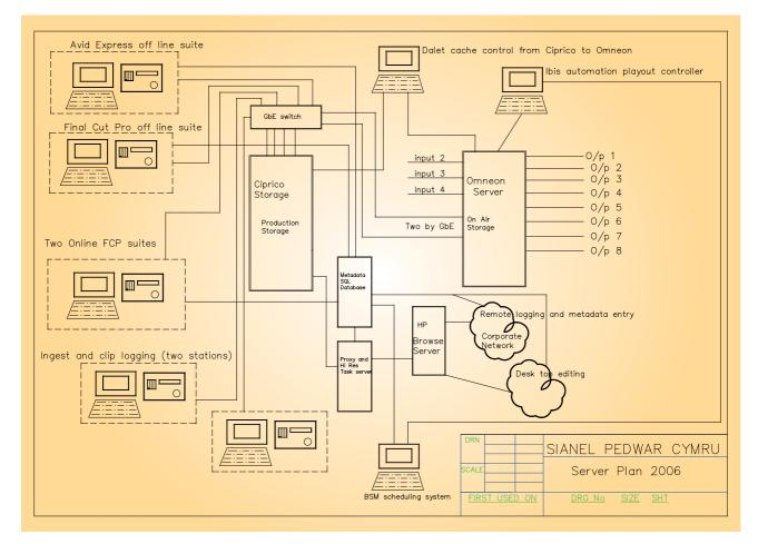
Linked to the Production storage are two off-line edit suites, an Avid and a Final Cut Pro (FCP), as well as two on-line suites, both FCPs. There are currently two PC-based ingest stations with an HP server providing low-resolution proxy storage.
