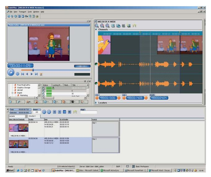
Clips selected in this way can be exported to the FCP suites directly from the client interface. This causes editing decisions made using low-resolution material to be mirrored in the high resolution part of the storage.
