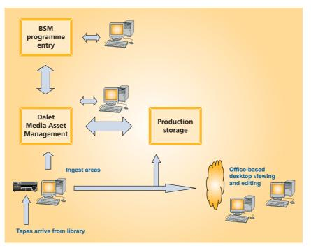
• The arrival of the DV files in the Dalet cluster triggers the generation of a low-resolution proxy file for desktop viewing and editing. This is typically a 400 kbit/s WMV (Windows Media) file.
