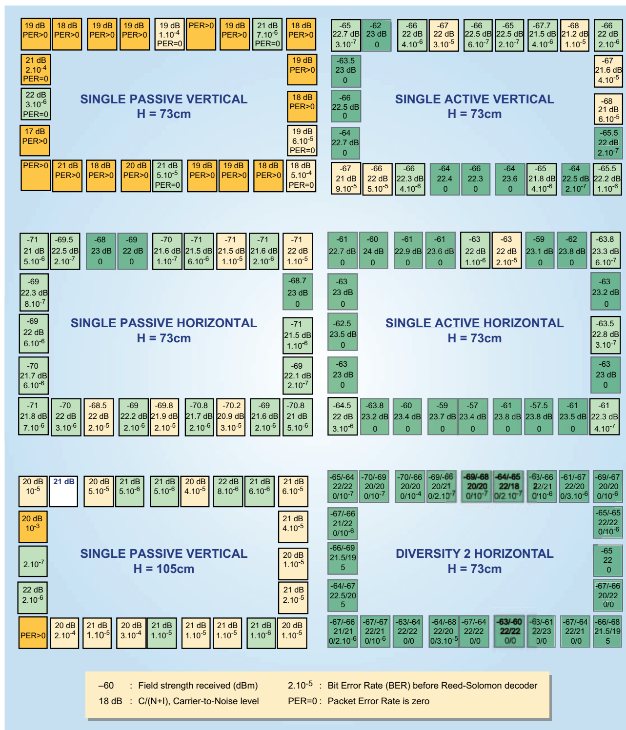
Figure 8 Comparison between different types of antennas and diversity reception in portable indoor situations: transmitter antenna polarization = horizontal
