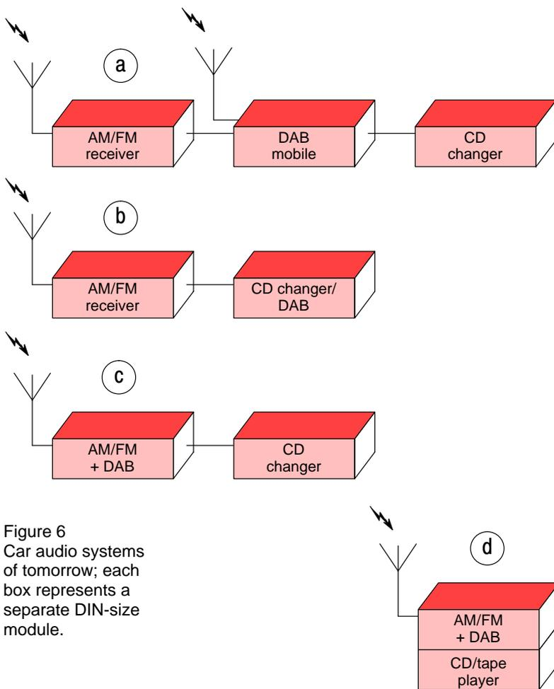
Figure 6 Car audio systems of tomorrow; each box represents a separate DIN-size module.
