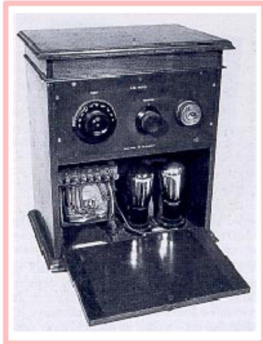
Figure 8 The Baby Grand AC-mains table model, made by Gambrell Brothers Ltd. in 1926.
