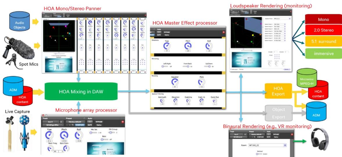
Figure 5: An example of a 3D audio production workflow based on HOA and the Qualcomm® 3D Audio tools suite [30]
