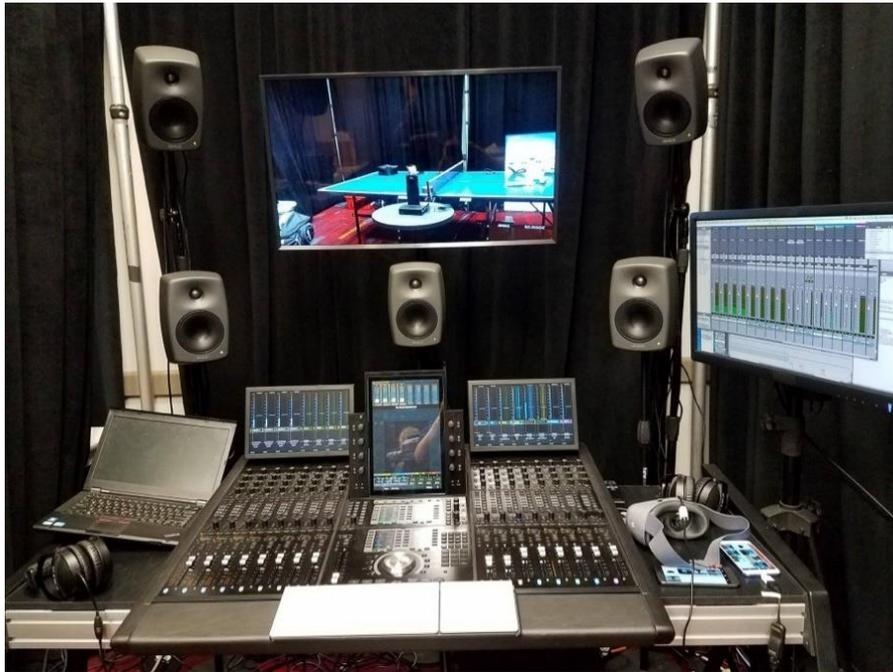
*Figure 6: An example of a monitoring system for the simultaneous production of SBA for VR and linear TV content. The workstation features a 7.1.4 loudspeaker system, an HMD for VR monitoring, and a DAW.*
