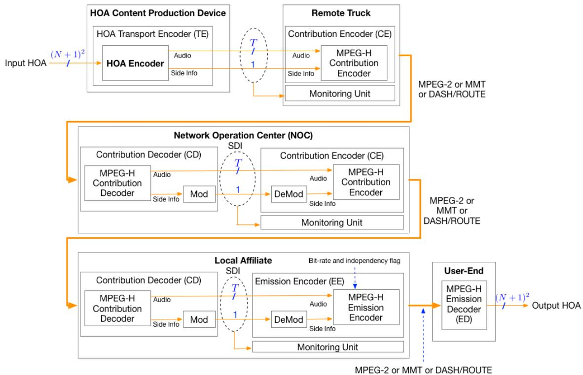
Figure 9: Workflow for the transport of HOA within existing broadcast facilities
