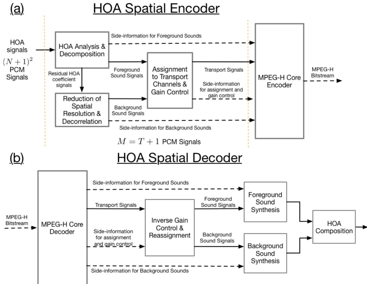
Figure 8: Block diagrams of a possible HOA Spatial Encoder (a) and the MPEG-H HOA Spatial Decoder (b) [5].
