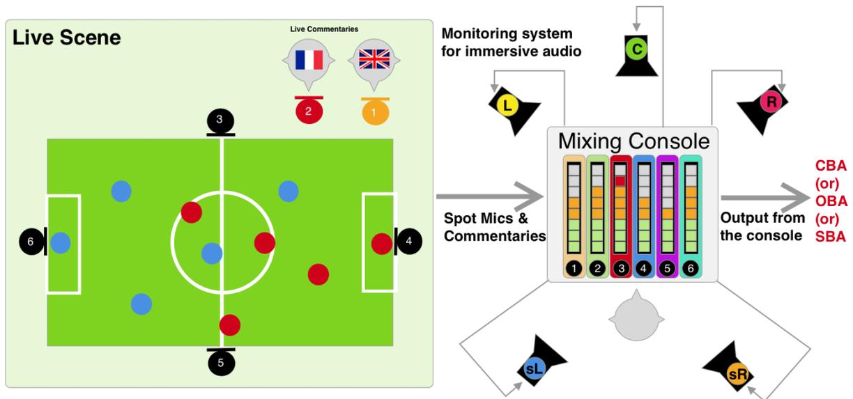
Figure 1: Live event with multiple microphones; the mixing engineer's environment
