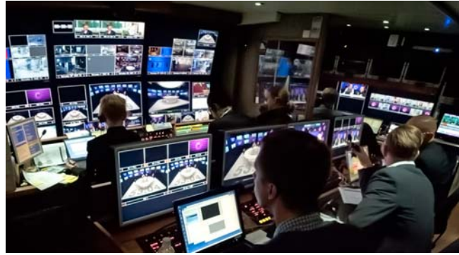
Four graphics operators in the OB truck during the last Swedish election, manning the multiple graphics outputs for real-time election data output by CasparCG (photo by Jonas Hummelstrand)
