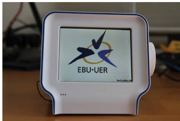
Figure 9 Chumby One displaying a RadioVIS service associated with FM
