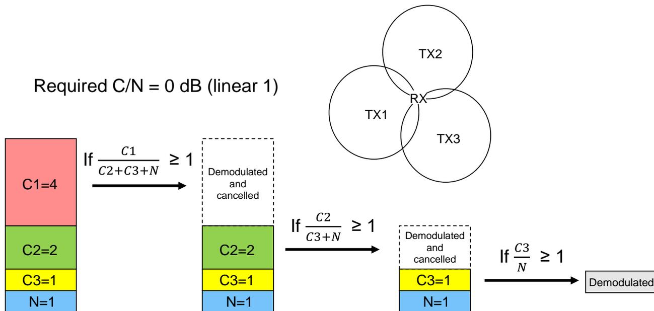
**Figure 3: Example of SIC; the weakest Tx3 signal (received with power C3) is demodulated in three steps**
