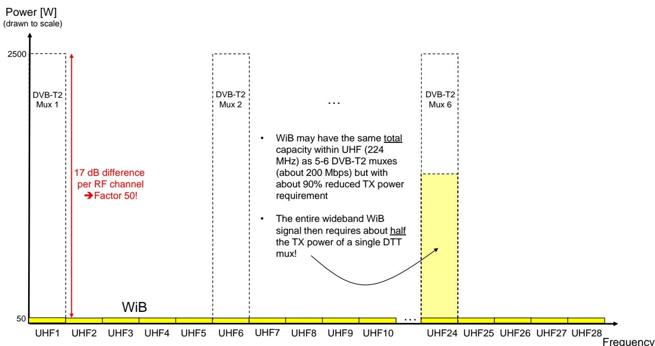
**Figure 1: Required power for DVB T2 and WiB**
