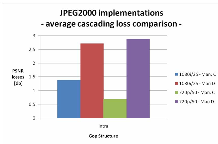
Figure 9: JPEG2000 average cascading losses
