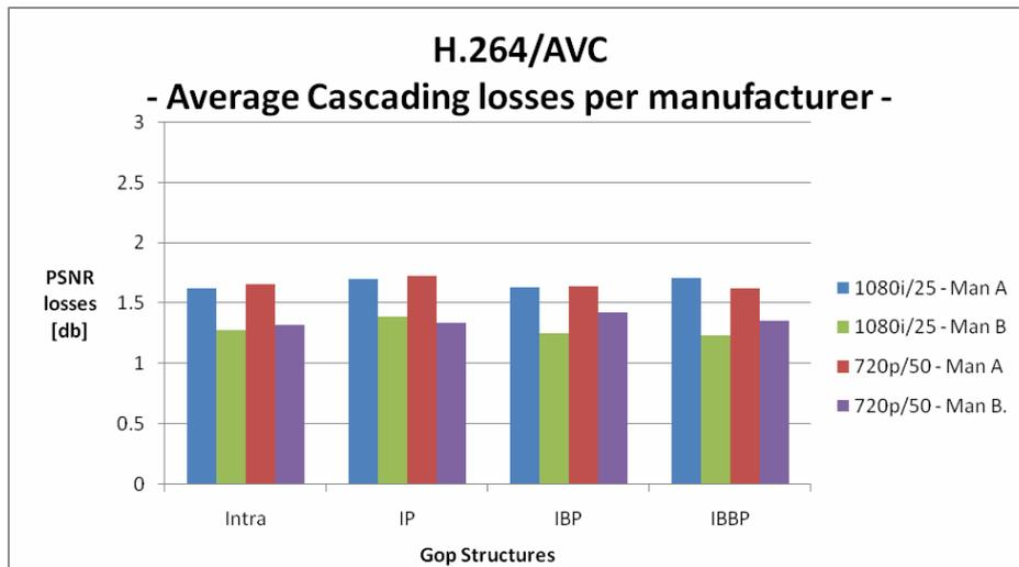
Figure 6: H.264/AVC average cascading losses per manufacturer
