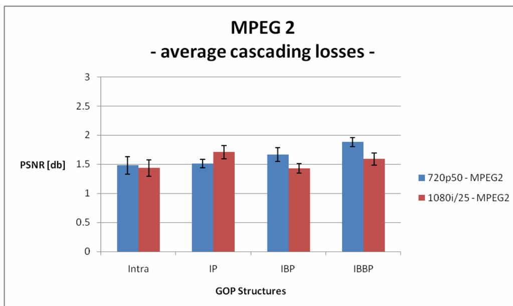
Figure 12: MPEG-2 average cascading losses
