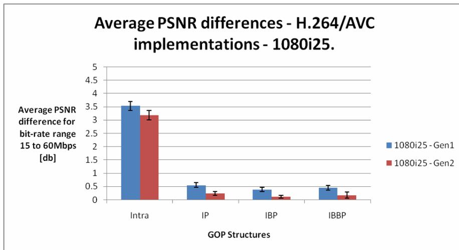
Figure 4: H.264/AVC implementation differences with 1080i/25 coding
