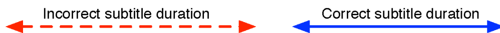
Figure 2: The potential temporal display errors that could be introduced by frame-based subtitle time quantisation.
