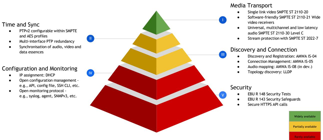
**Figure 1: Minimum user requirements to build and manage an IP-based media facility**
