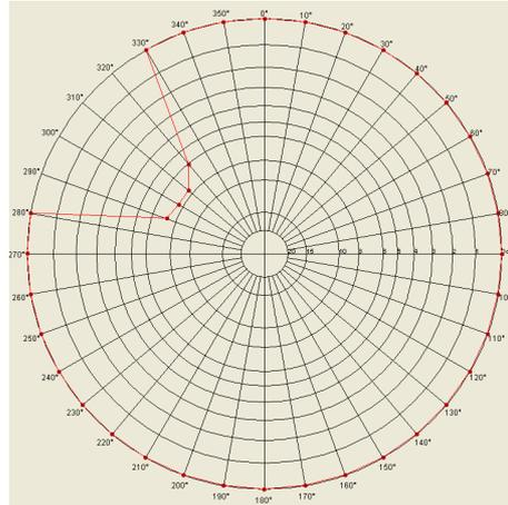
Figure E10: Radiation patterns of the new DRM+ transmitter Giessen 99.2 MHz
