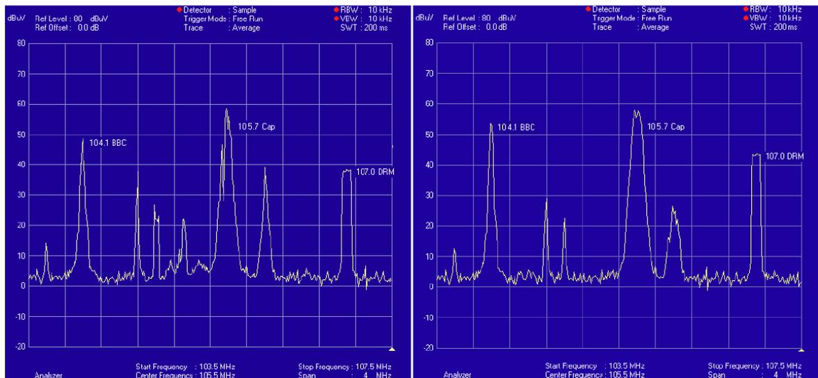
Figure G14: Spectrum plots taken at North Queensferry (left) and Leith Docks (right) showing BBC Radio nan Gaidheal, Capital FM and the DRM signal
