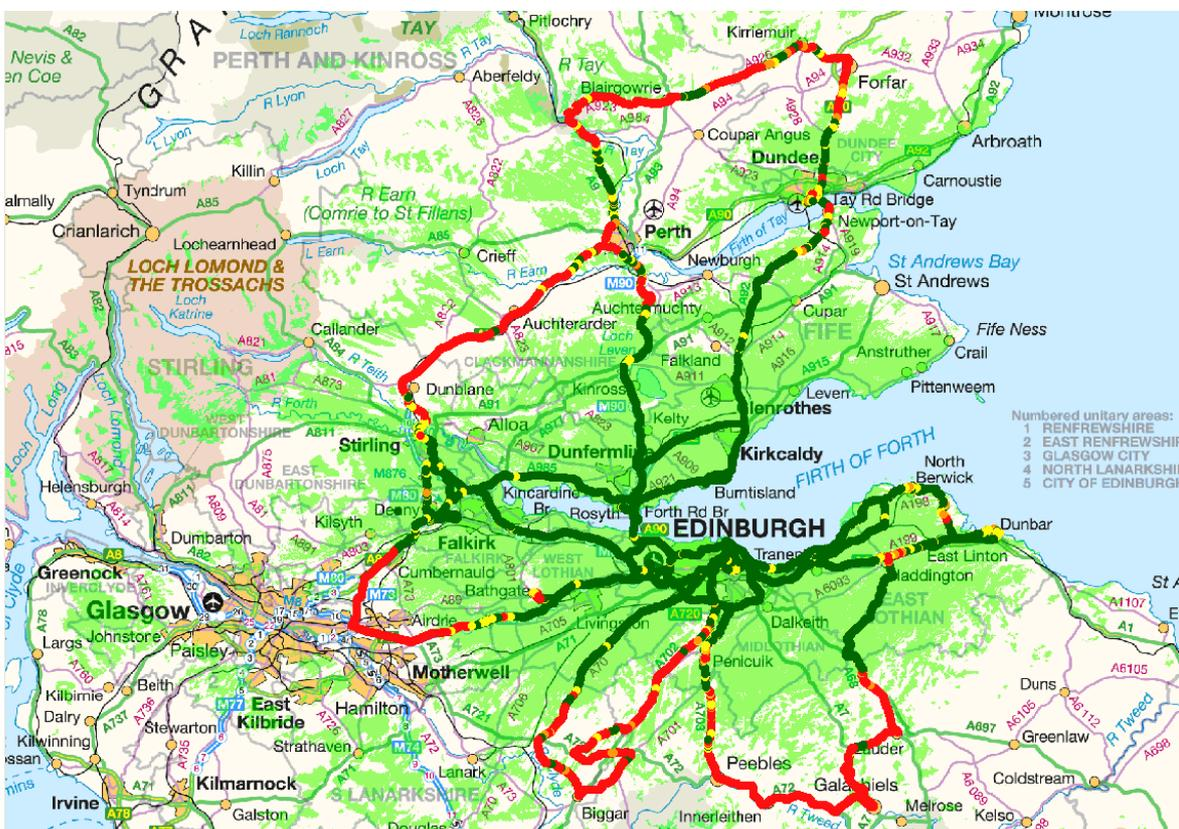
Figure G15: Overall coverage, 4-QAM rate 1/3.
