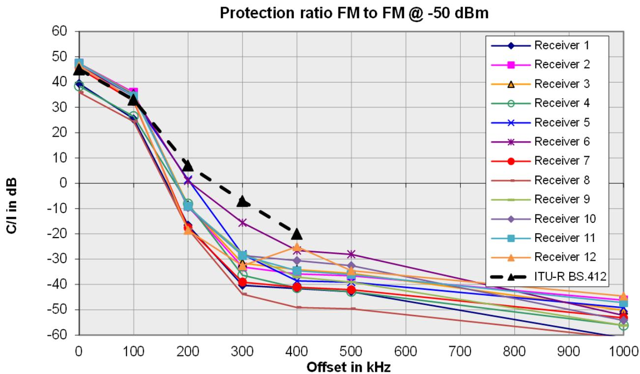
Figure F2: Measured protection ratios for FM interfered by FM; 12 hifi tuners
