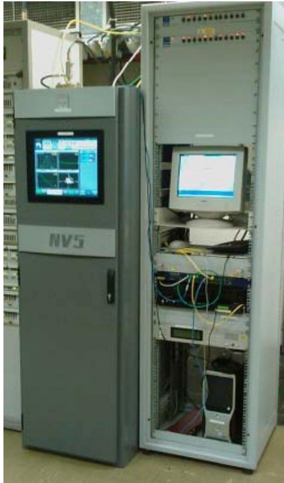
Figure G7: The DRM+ transmitter (left) and content server, modulator and monitoring receiver (right)
