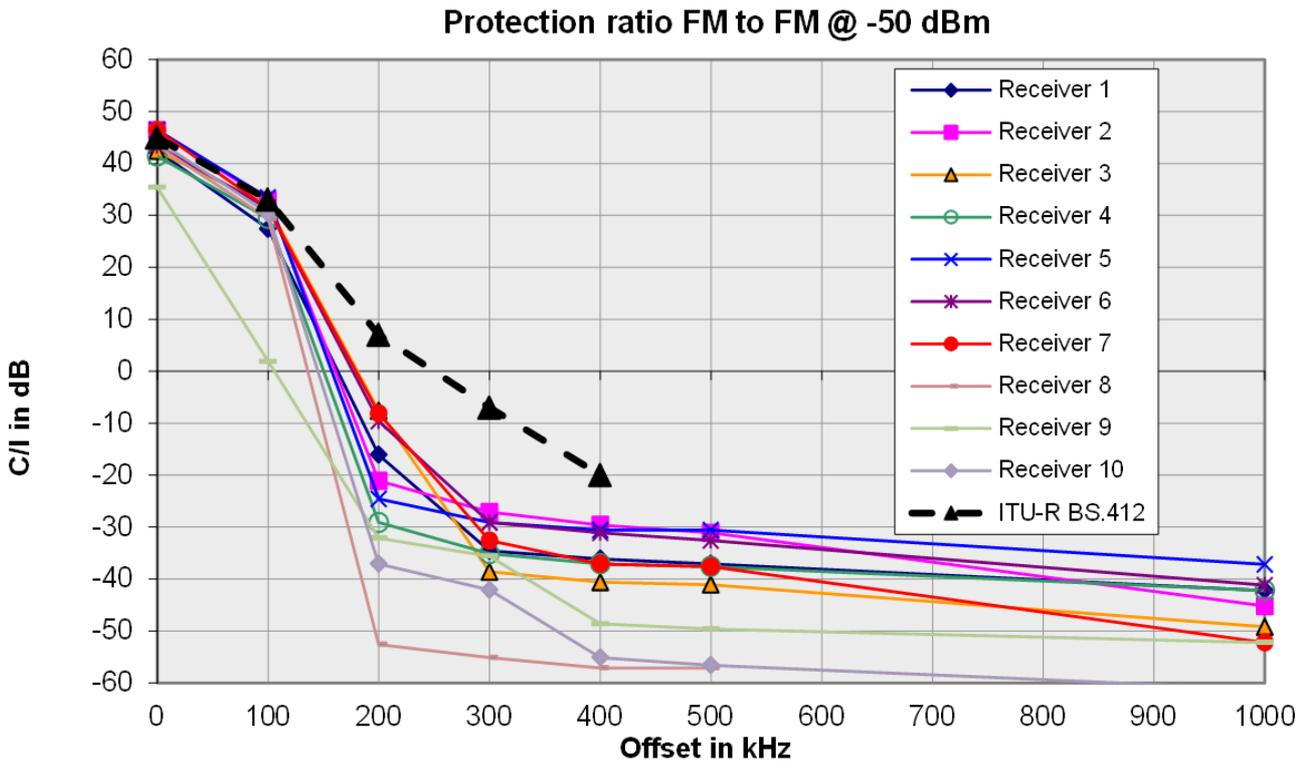
Figure F5: Measured protection ratios for FM interfered by FM; 10 car receivers
