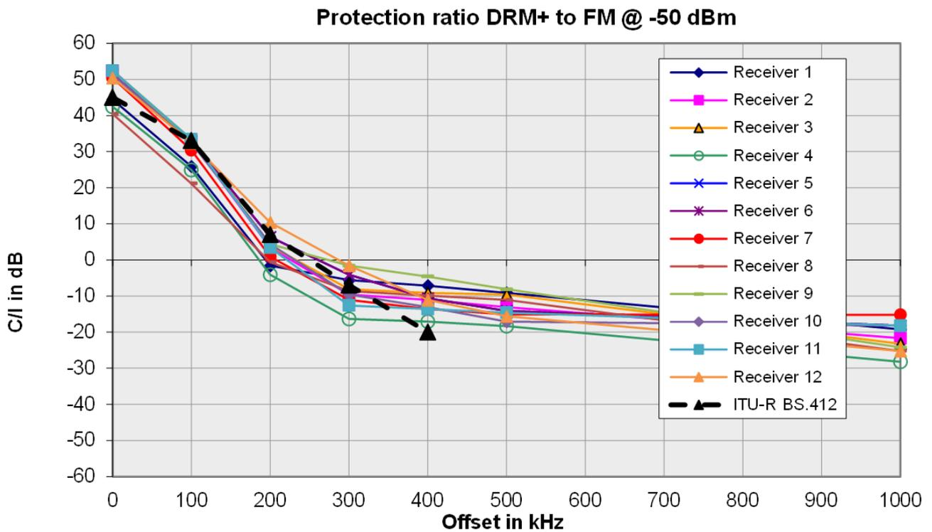
Figure F3: Protection ratios for FM interfered with OFDM (hifi tuners)
