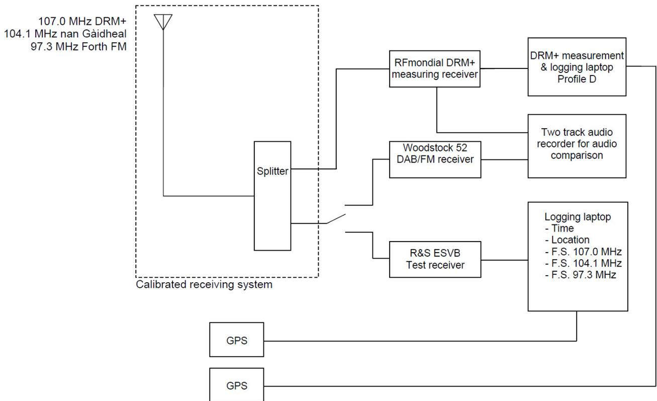
**Figure G10: Receiver equipment schematic**
