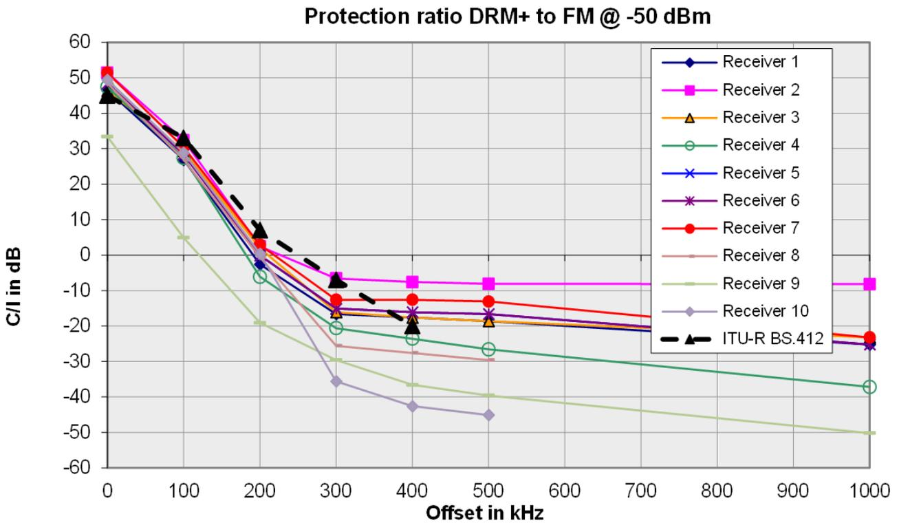
Figure F6: Protection ratios for FM interfered with OFDM (car receivers)
