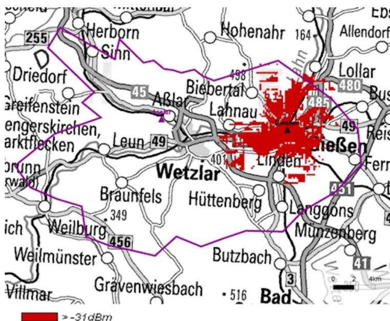
Figure E15: Interference contour of FM transmitter Asslar 100.5 MHz
