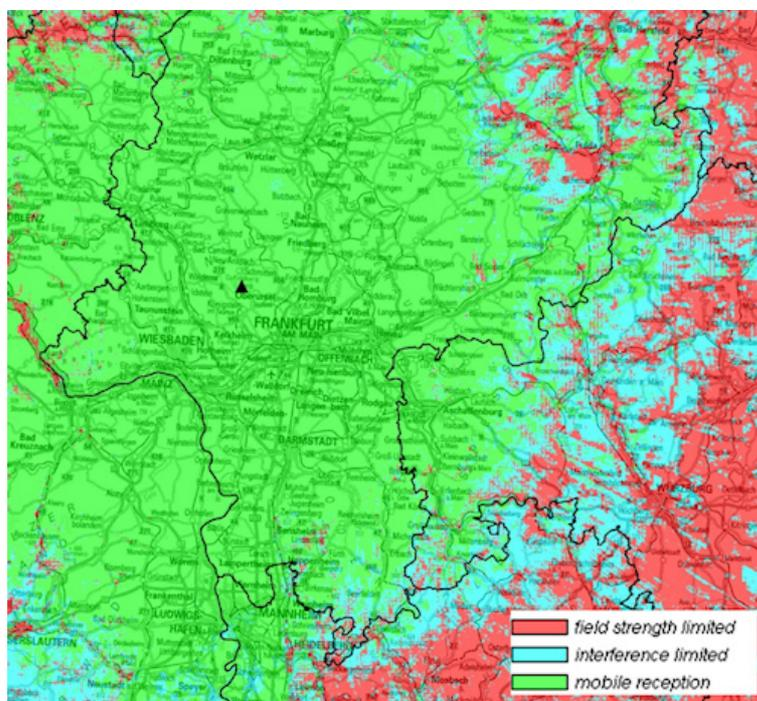
Figure D3: DRM+ mobile reception (4-QAM 1/3)
