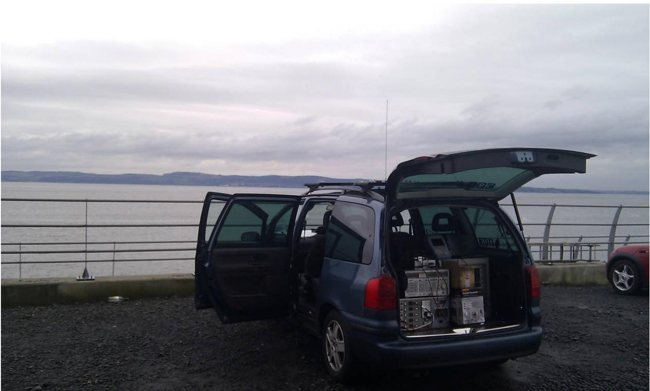
Figure G9: BBC Measuring vehicle
