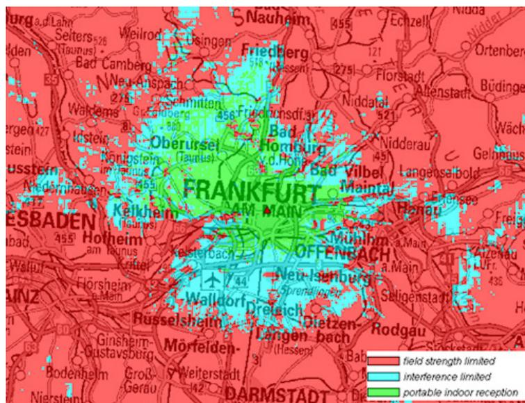
Figure C5: DRM+ portable indoor reception (4-QAM 1/3)
