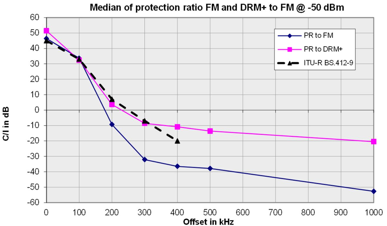
Figure F4: Median protection ratios for analogue and digital interferer (hifi tuners)
