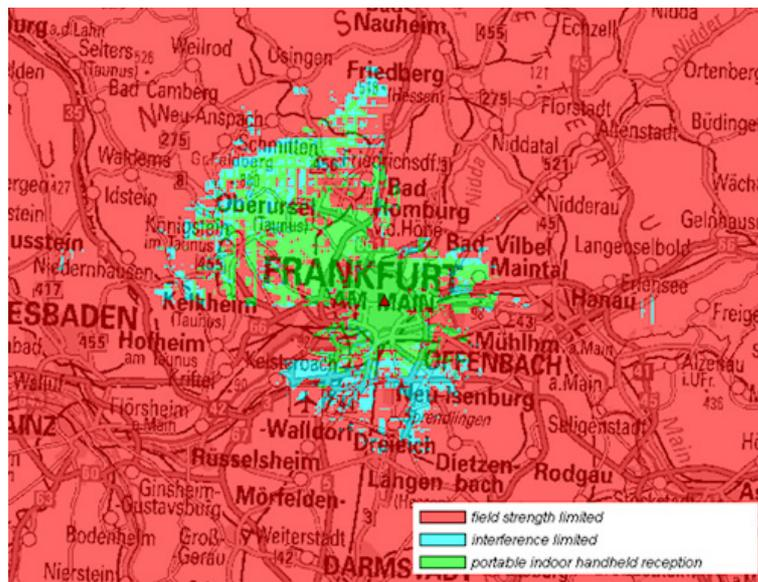
Figure C6: DRM+ portable indoor handheld reception (4-QAM 1/3)
