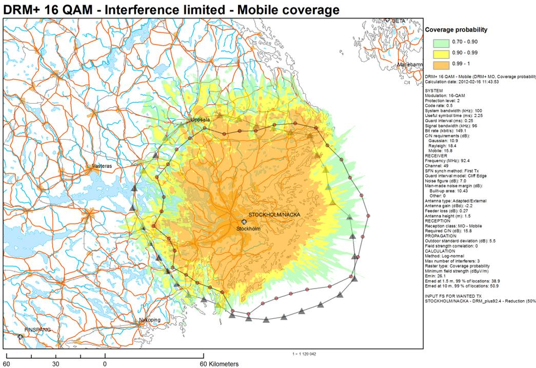
Figures B5 & B6: Coverage contour and pixel based coverage for DRM+ Transmitter QPSK 1/3 and 16-QAM Mobile reception. Population Coverage is 2.020 and 1.936 millions, resp.
