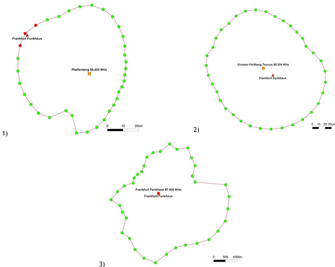
Figure C3: DRM+ transmitter and FM interference contours
