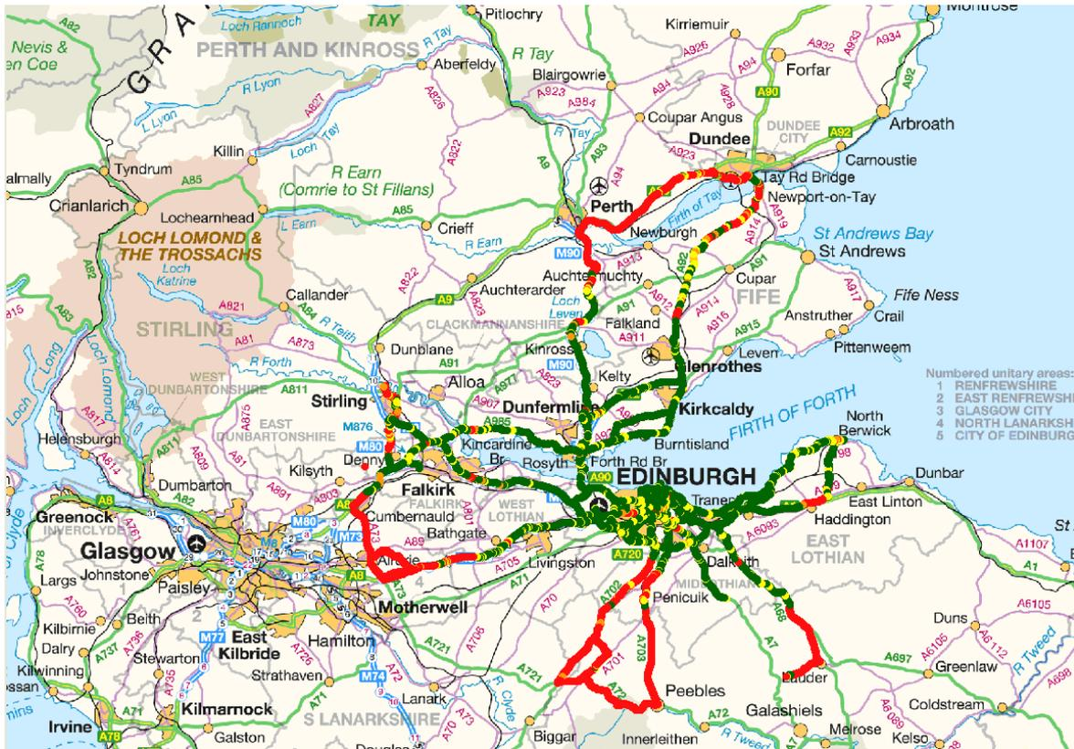
Figure G16: Overall coverage, 16-QAM, rate 1/2
