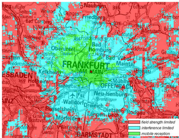
Figure C4: DRM+ mobile reception (4-QAM 1/3)
