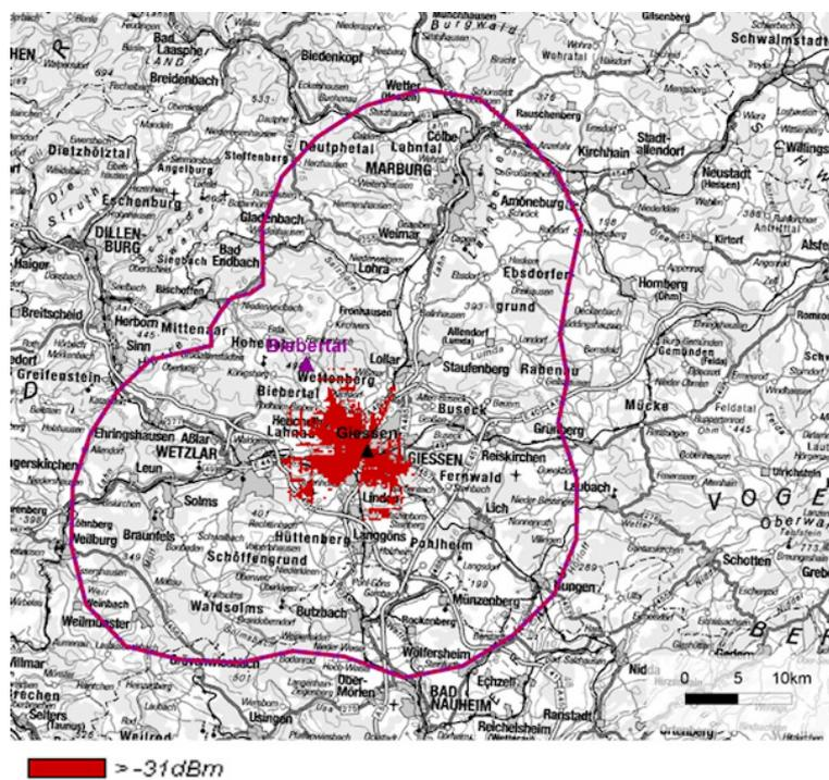
Figure E7: Interference contour of FM transmitter Biebental 92.6 MHz
