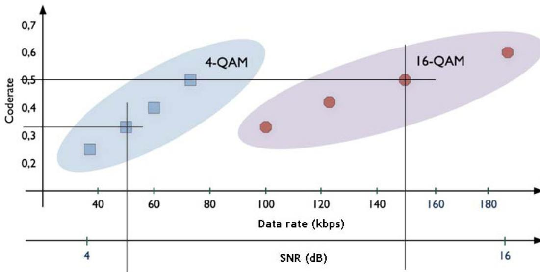
Figure G17: Comparison of data rate and required SNR in a Gaussian channel for different constellations and code rates
