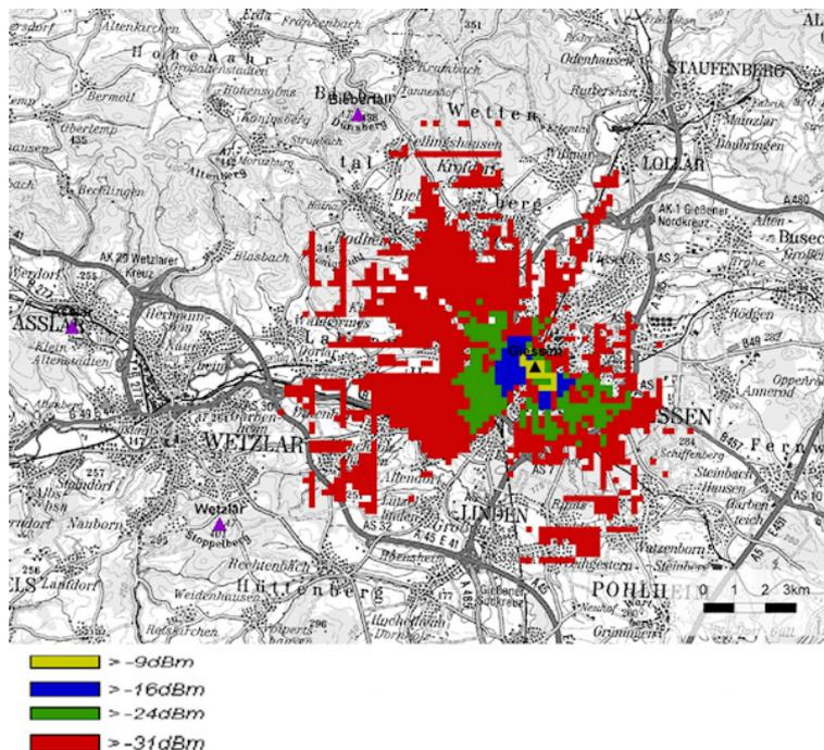
Figure E6: Regions potentially affected by cross-modulation
