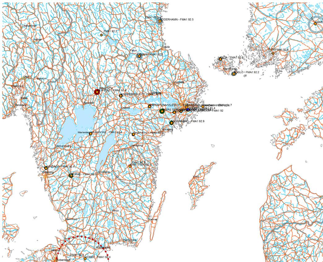
**Figure B2: The victim transmitters found when converting from FM into DRM+.**
