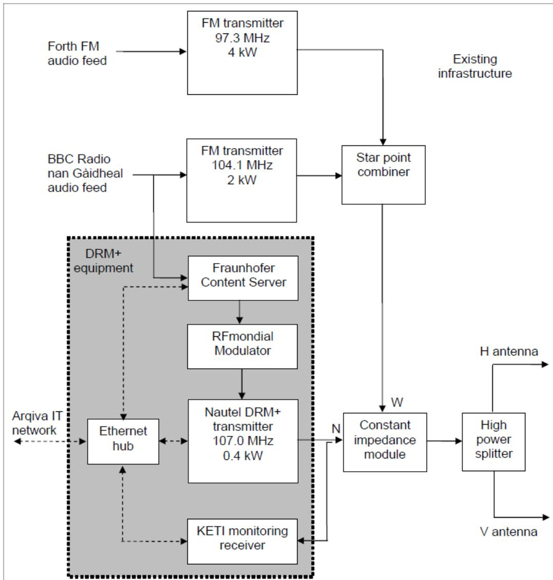
Figure G6: Block diagram of transmission system (simplified) showing existing infrastructure and additional DRM+ equipment
