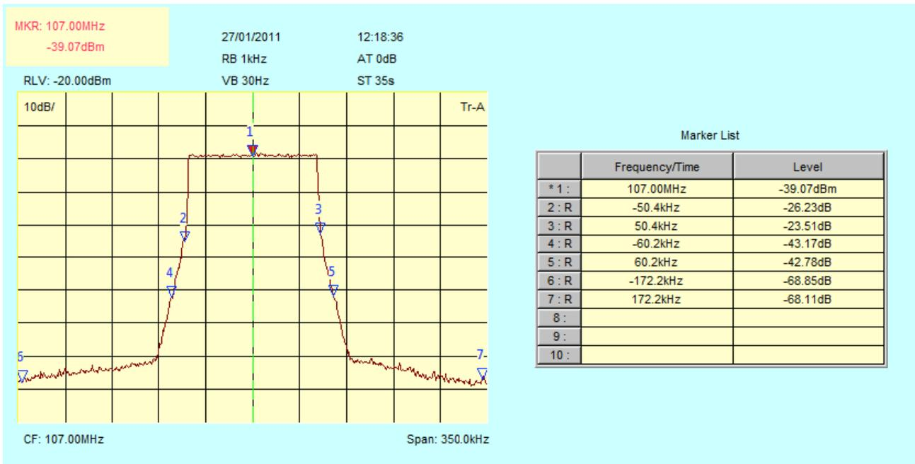
Figure G8: Recorded spectrum of DRM+ signal
