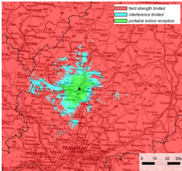
Figure E12: DRM+ portable indoor reception (4-QAM 1/3)
