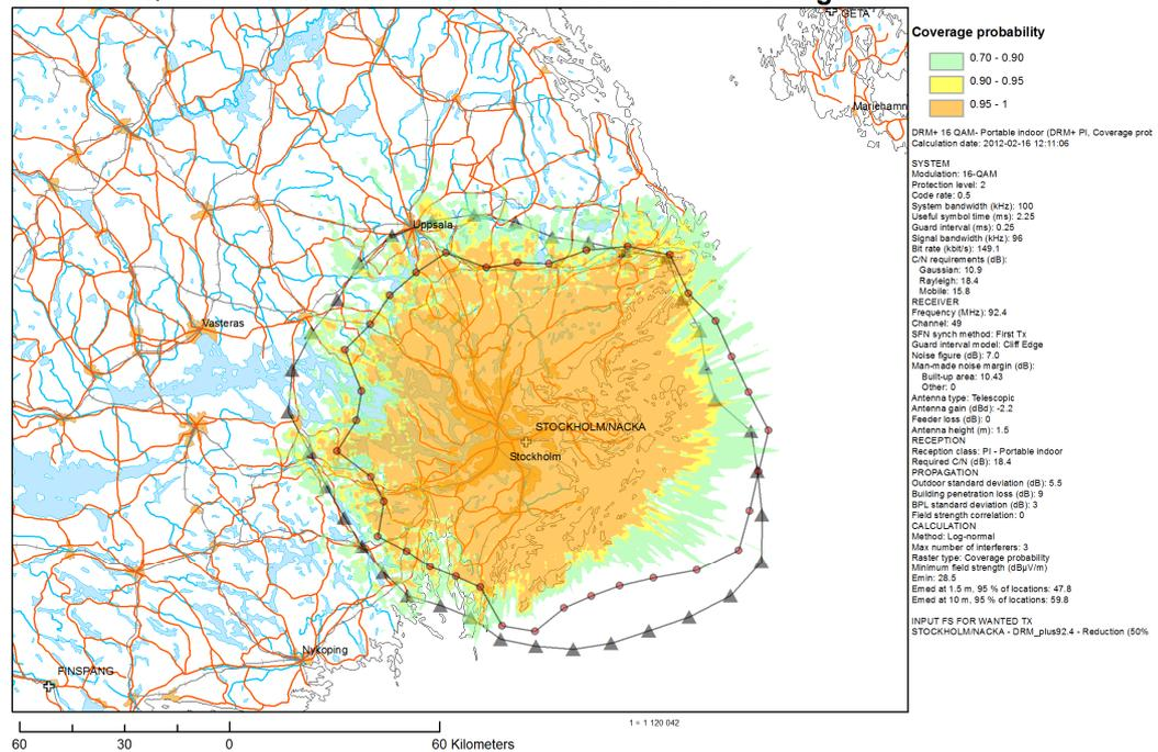
Figures B7 & B8: Coverage contour and pixel based coverage for DRM+ Transmitter QPSK 1/3 and 16-QAM Portable Indoor Coverage. Population Coverage is 1.980 and 1.861 millions, resp.
