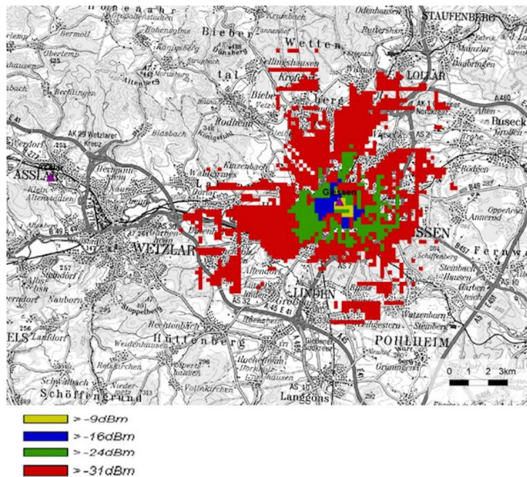
Figure E14: Regions potentially affected by cross-modulation
