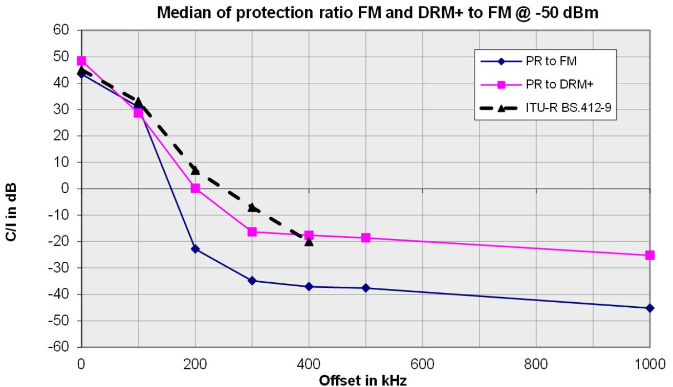
**Figure F7: Median protection ratio for analogue and digital interfering signal (car receivers)**
