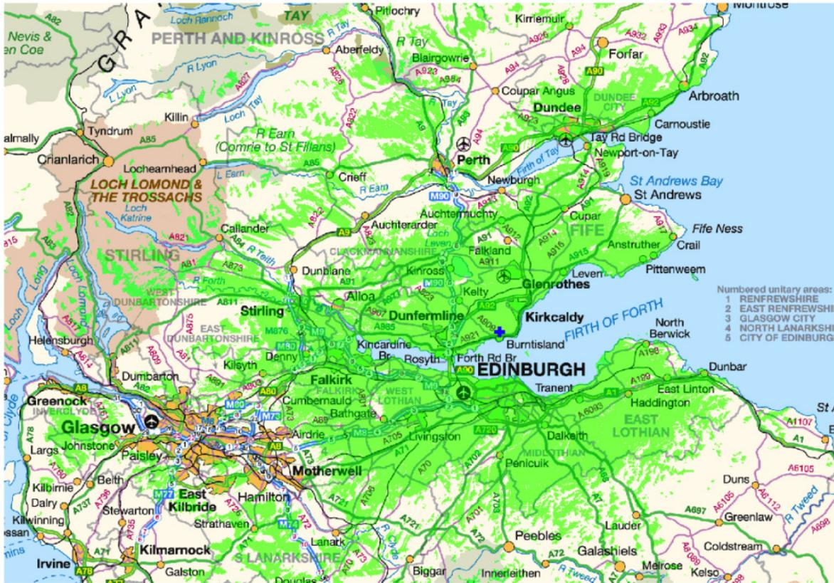
Figure G11: Predicted coverage area for a 1kW DRM+, 4QAM, rate 1/3 station
