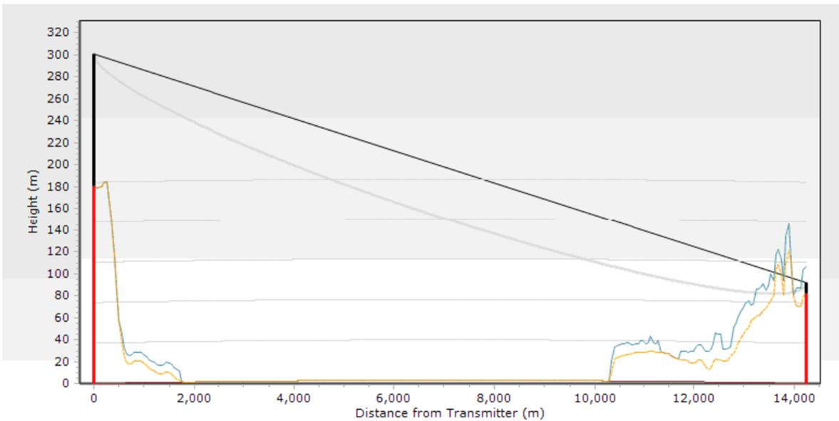
Figure G22: Path profile for light blue ring in Figure G20
