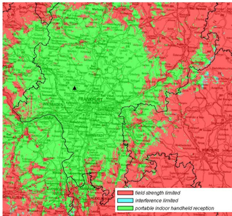
Figure D5: DRM+ portable indoor handheld reception (4-QAM 1/3)
