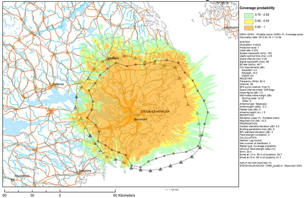
DRM+ 16 QAM - Interference limited - Portable indoor coverage
