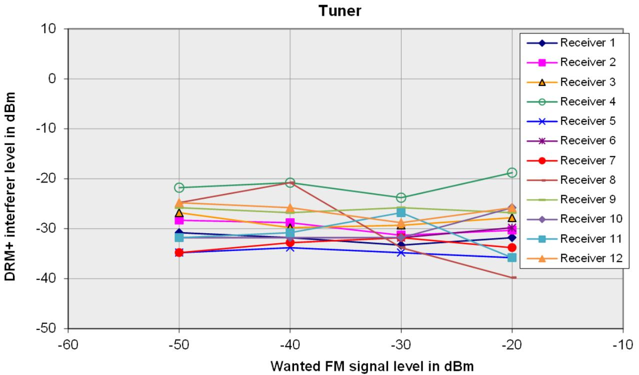
Figure F8: Allowable level of digital interfering signal vs. wanted FM signal level (hifi tuners)
