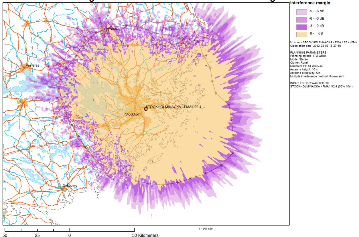
**Figure B2: Terrain based interference limited coverage and interference contour. The agreement between the two coverage areas is quite good.**
