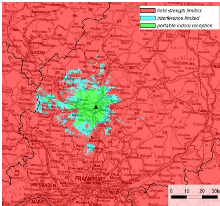
Figure E4: DRM+ portable indoor reception (4-QAM 1/3)
