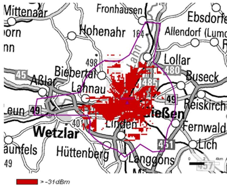
Figure E16: Interference contour of FM transmitter Giessen 97.9 MHz
