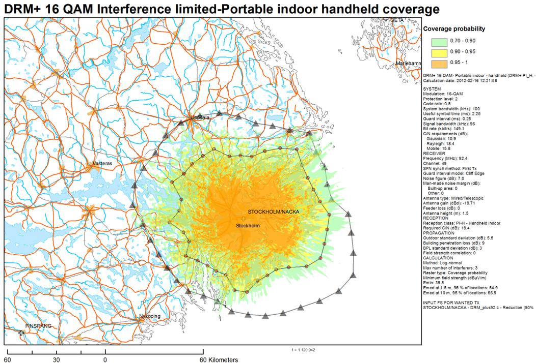
Figures B9 & B10: Coverage contour and pixel based coverage for DRM+ Transmitter QPSK 1/3 and 16-QAM Portable Indoor Coverage handheld. Population Coverage is 1.843 and 1.634 millions, resp.
