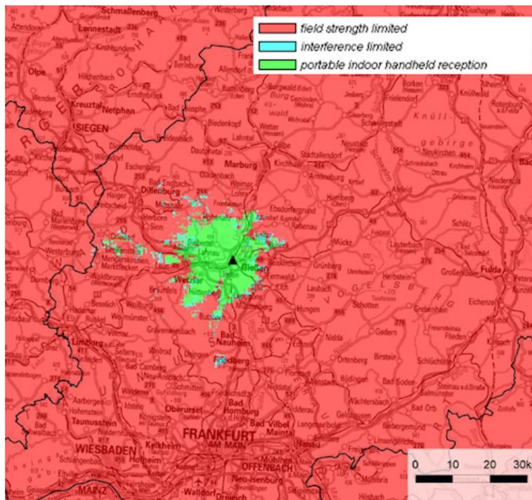
Figure E5: DRM+ portable indoor handheld reception (4-QAM 1/3)
