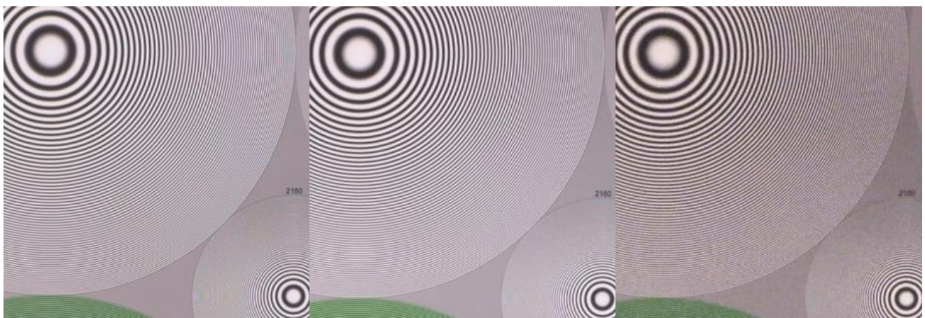
Figure 7 Resolution (HD 1920x1080): the effects of gain setting
