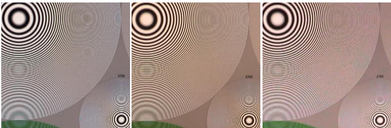
Figure 13 Softening with gain, HD, Look 1 Normal ISO 160 ISO 800 ISO 6400
