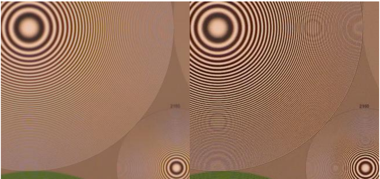
Figure 6 Zone plate, resolution at HD, Look 3, Neutral
