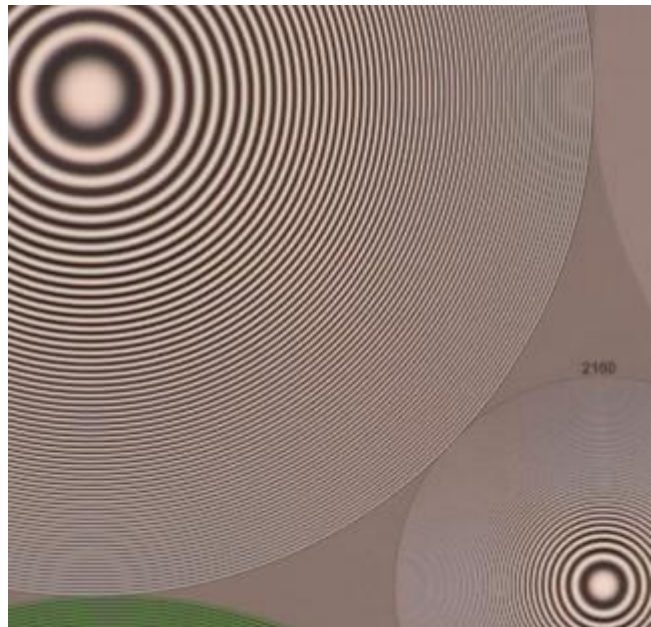
Figure 3 Zone plate, resolution HD, Look 3, Neutral
