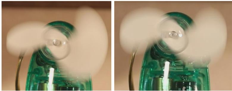
**Figure 13 Rolling shutter effect, HD and 4K**
