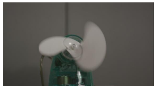
Figure 16: Rolling shutter effect
