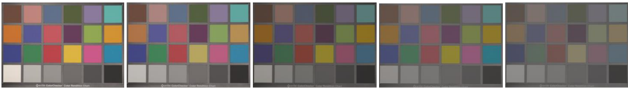
Figure 1: Colorchecker a: Preset off Normal 3 (BT.709) b: Preset BT.709 c: Preset Canon Log d: Preset Canon Log 2 : BT.709 e: Preset Canon Log 2 : C.Gamut
