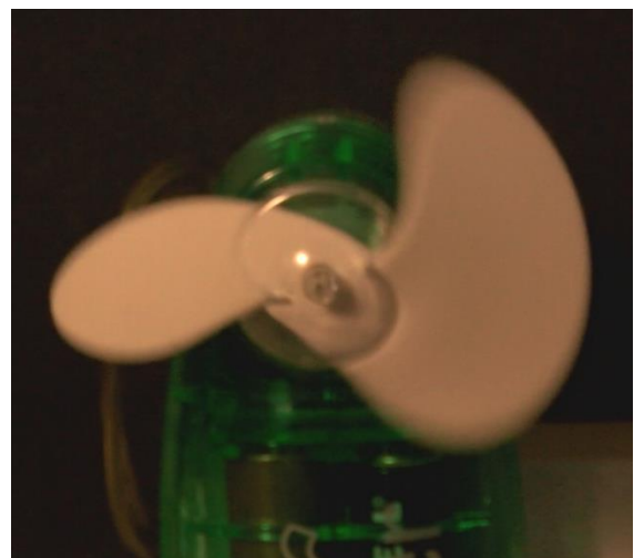
Figure 12 Rolling shutter, fan
