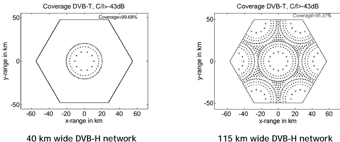
Figure A4.2: Service coverage of the DVB-T network in the presence of DVB-H interfere on an adjacent channel.
