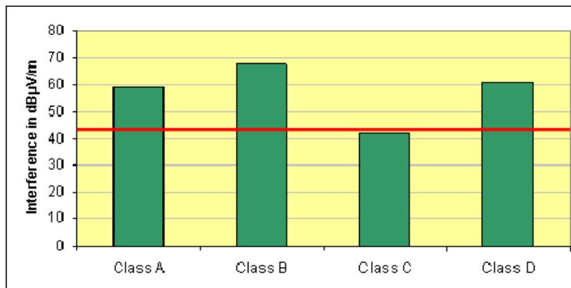
Figure 7.5. The interference field strength of a DVB-H network (system variant 16 QAM 2/3) in comparison with the interference potential of the reference network RN1 RPC2 at 500 MHz.
