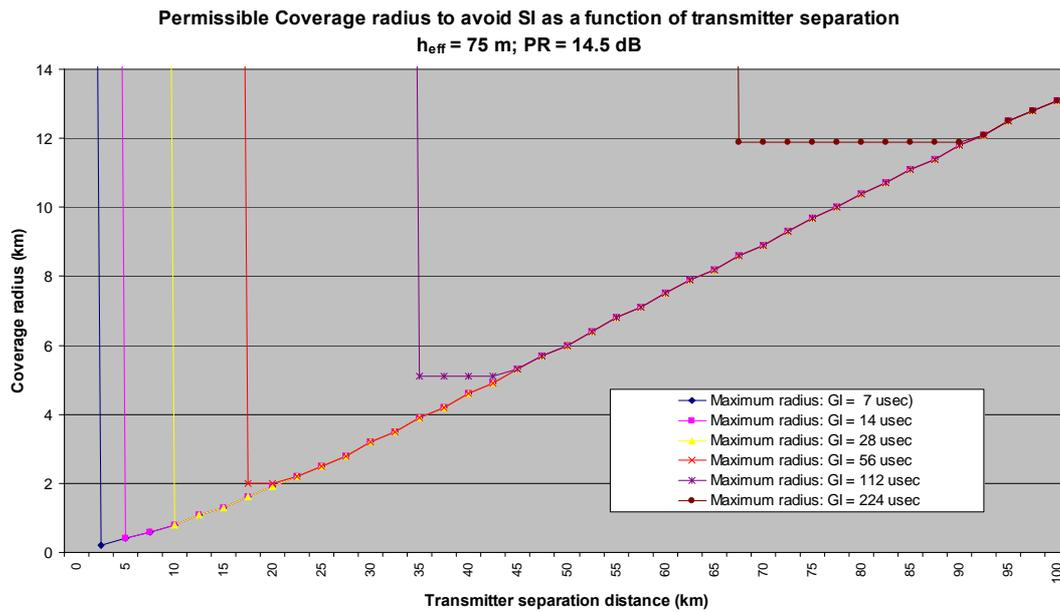
Figure 5.1: Coverage radius to avoid self-interference.
