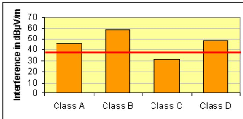
Figure 7.3: The interference field strength of the four T-DMB classes in comparison with the interference potential of the reference network RN RPC5.
