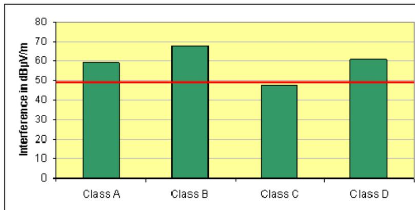
Figure 7.6. The interference field strength of a DVB-H network (system variant 16 QAM 2/3) in comparison with the interference potential of the reference network RN1 RPC2 at 800 MHz.
