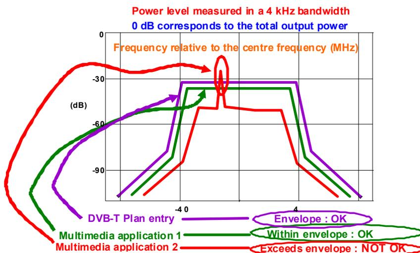
Figure 7.1. Interference envelope concept of the GE06 Agreement.
