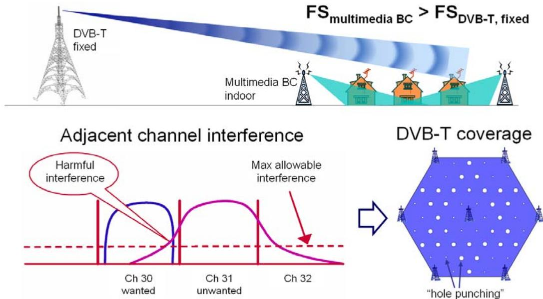
Figure 5.2: Adjacent channel interference from DVB-H broadcasting network into DVB-T service
