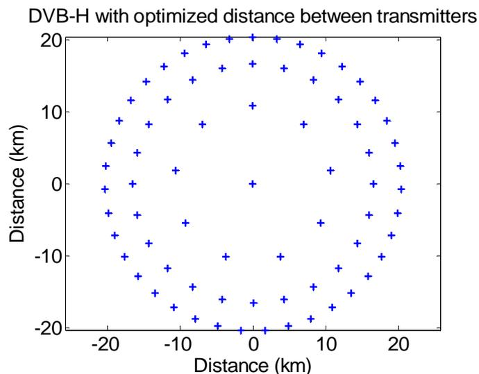
Figure A4.1: Optimised locations (blue crosses) of DVB-H transmitters in the network.
