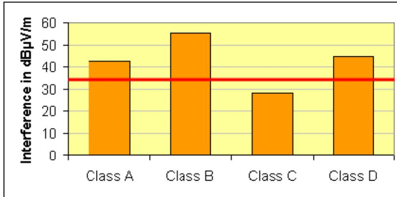
Figure 7.4: Interference field strength of four T-DMB blocks in comparison with the interference potential of the reference network RN1 RPC2
