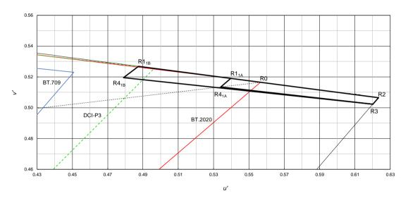
Figure 3: CIE u'v' diagram of red primary tolerances
