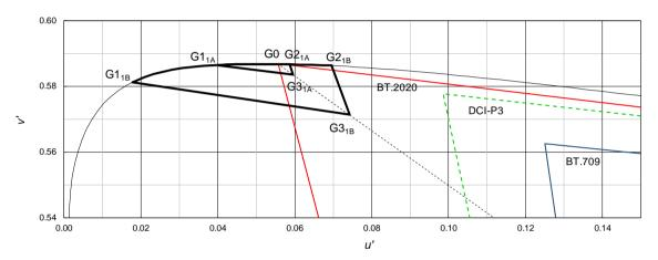
Figure 5: CIE u'v' diagram of green primary tolerances
