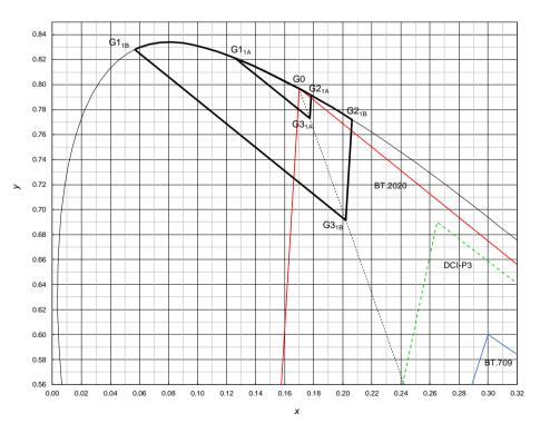
Figure 6: CIE xy diagram of green primary tolerances
