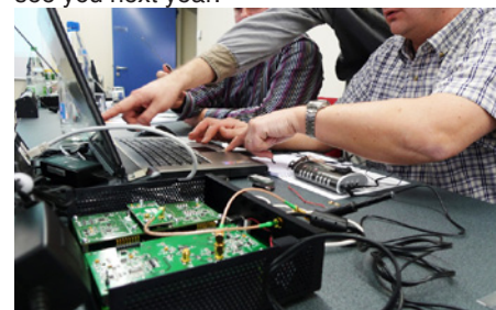
Participants from Teleko (Czech Republic) producing an L band DAB transmission using CRC mmbTools on their laptop and a Universal Software Radio Peripheral (USRP black box at the front).
