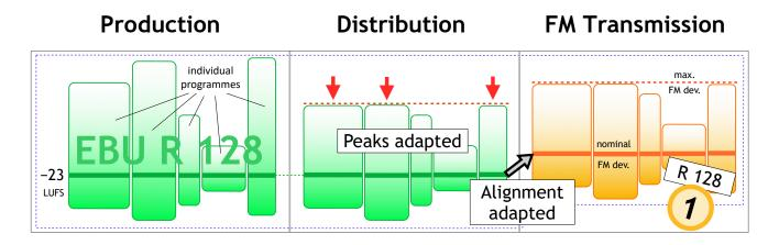
Figure 1: Levelling Scheme for a Radio station using R 128 compliant loudness normalisation at
