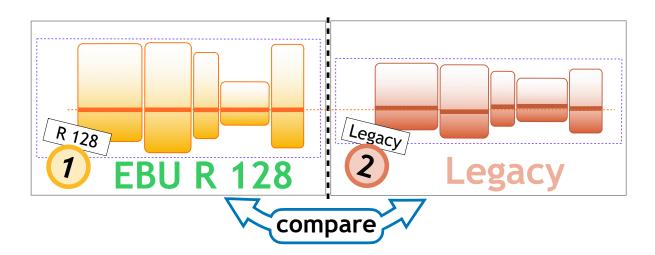
Figure 3: Comparison between the results of an FM Levelling Scheme according to EBU R 128 and of a legacy method (R 128 1 vs. Legacy 2). The same loudness level is achieved, but R-128-compliant loudness normalisation reduces transmission processor aggressiveness and enables a more dynamic, open sound
