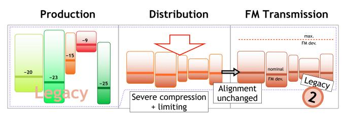
**Figure 2:** Levelling Scheme for a Radio station using no normalisation in production with legacy processing and alignment for FM. The resulting average loudness is the same as in Fig.1. Severe peak limiting and compression lead to a less dynamic, more squashed sound (Legacy 2).
