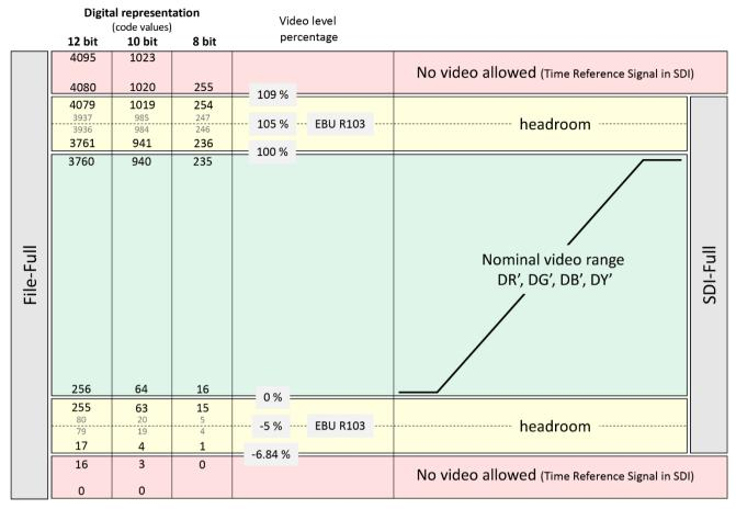
Figure 1: Typical signal levels for SDI
